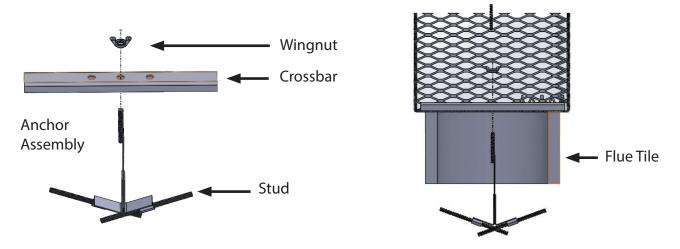
3. Place base screen onto flue tile. Screw studs out until they touch the flue walls, then back off each stud about 1/2 to 3/4 of a turn. The anchor should hang freely with about 1/8" space between the tips of the studs and the flue wall.
