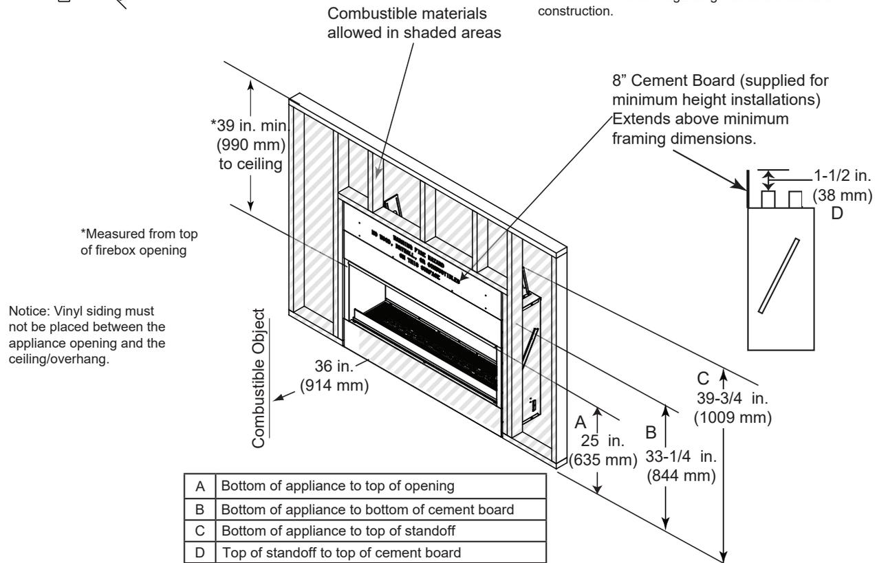
Figure 3.2. Appliance Locations and Framing Dimensions - ODLANAIG-48
