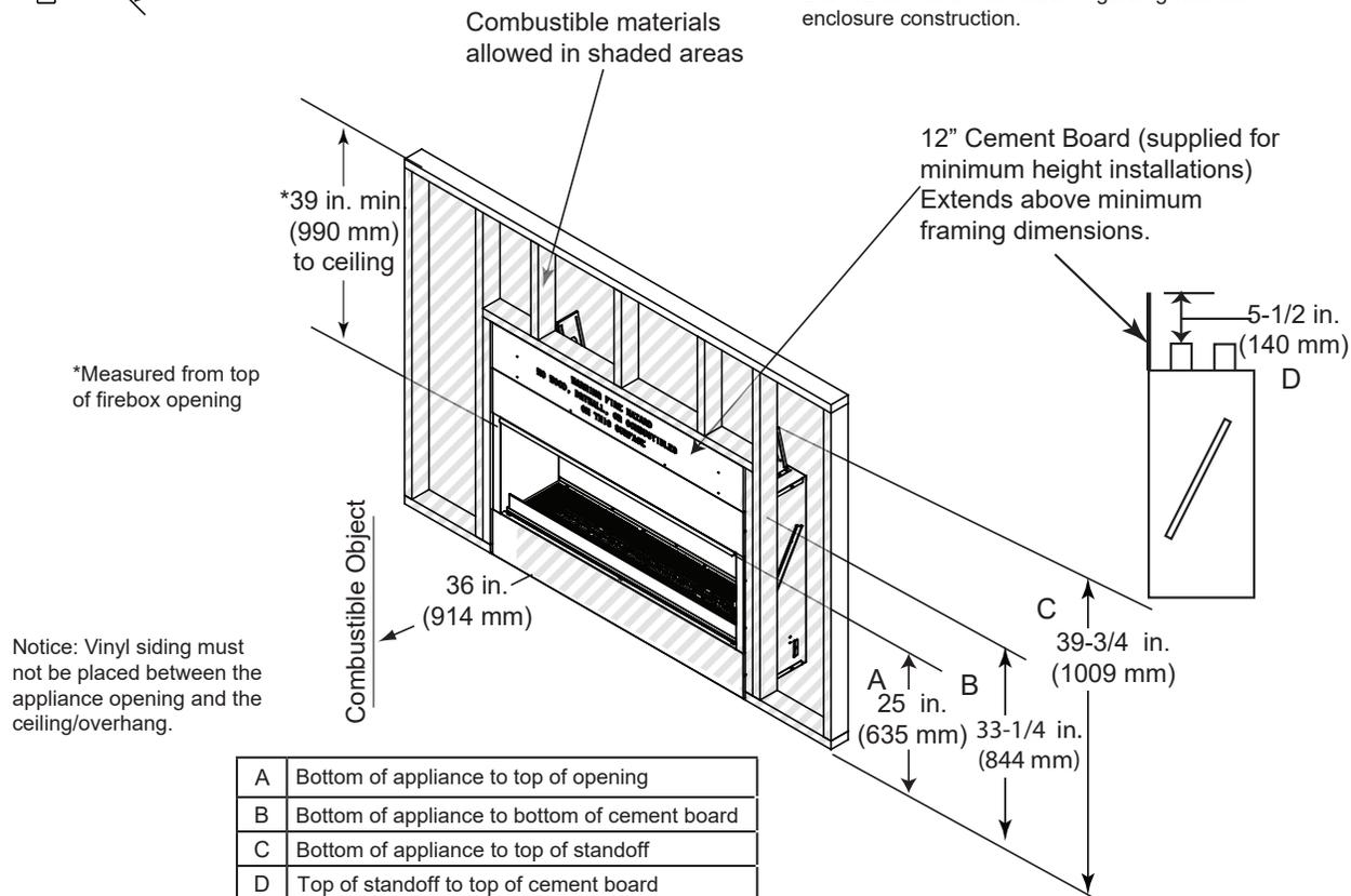
Figure 3.3. Appliance Locations and Framing Dimensions - ODLANAIG-60
