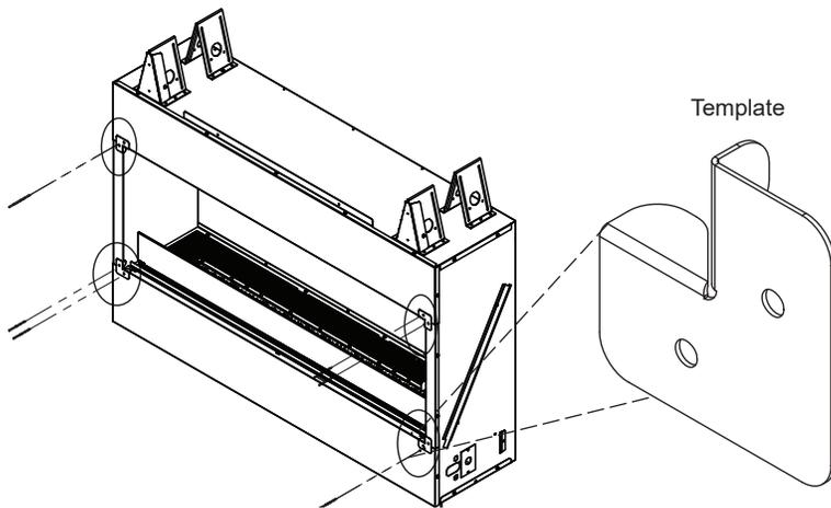
**Figure 2.** Install The top bottom and side trims
