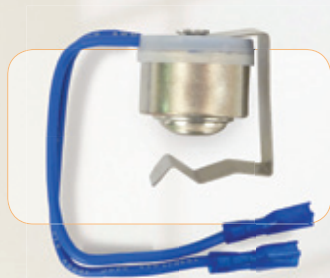
The optional aqua stat component makes sure the water temperature is over 115° before the fan is turned on.
