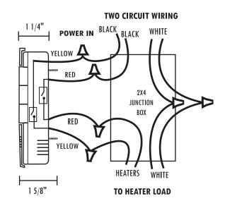
NOTE: When wiring verify proper phase with a voltmeter for each circuit.
