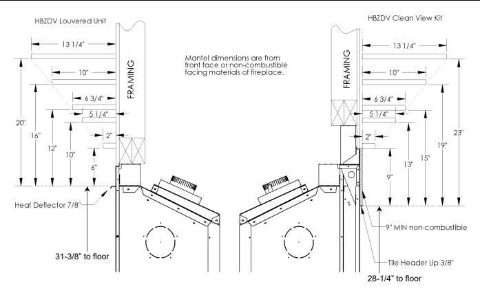
**Warning:** Combustible objects must not be placed on a non-combustible mantel unless the non-combustible mantel meets the minimum height and width requirements for a combustible mantel.
