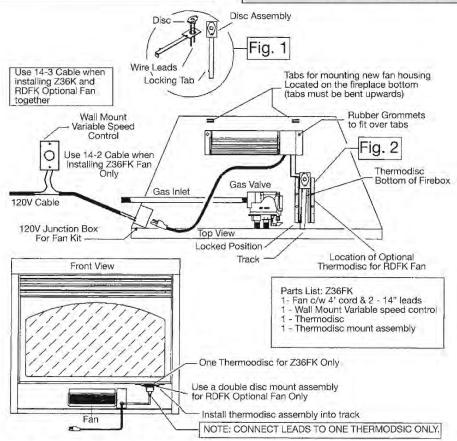
CAUTION - DO NOT ATTACH 120V FAN ASSEMBLY TO MILLIVOLT GAS VALVE SYSTEM
