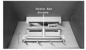
**STEP 1:** Remove the 2 grate bar screws and remove the grate bar.
