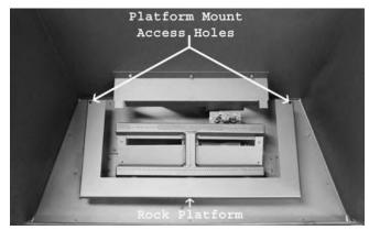
**STEP 3**: Using the rock platform mount holes, attach the rock platform to the burner pan as shown.
