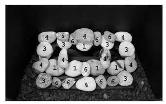
Finished Rock F3 Setup Never place any of the rocks directly onto the burner tubes.
