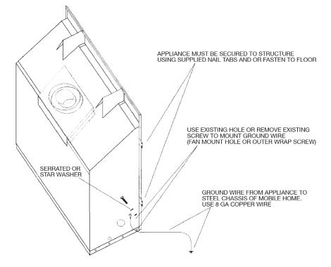
THE HBZDV3628N/NE/NE2 & HBZDV3628LP/LPE/LPE2 MAY BE INSTALLED IN MANUFACTURED (MOBILE) HOMES AFTER FIRST SALE IN THE USA. IN CANADA THE HBZDV3628N/NE/NE2 & HBZDV3628LP/LPE/LPE2 MAY BE INSTALLED IN MANUFACTURED (MOBILE) HOMES.
