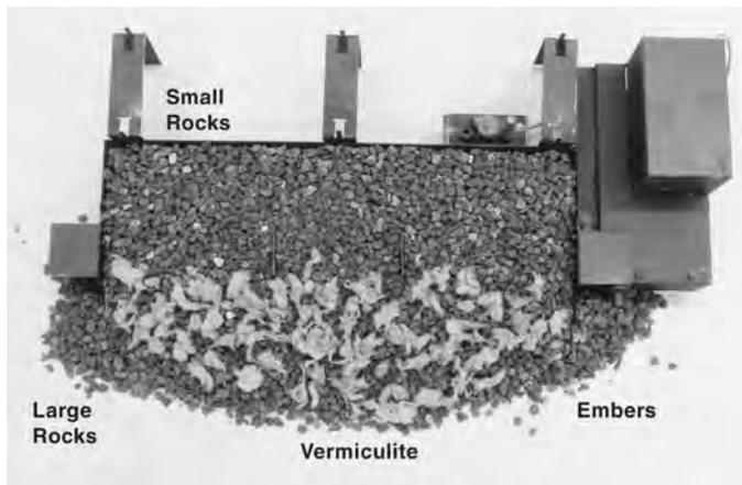
Place silica sand (NG only) or 1/4" small rock (LP only) inside and in front of burner pan. Place 1" large rock inside, in front, and around the sides of the pan. Place rock wool in front of center log support as shown. Sprinkle vermiculite over top of lava rock and rock wool.
