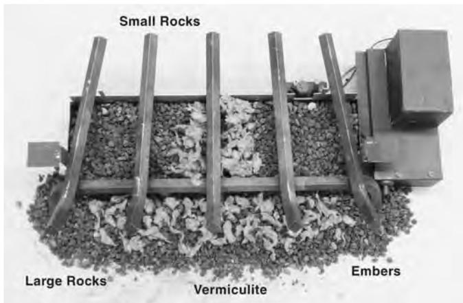
Place silica sand (NG only) or 1/4" small rock (LP only) inside and in front of burner pan. Place 1" large rock inside, in front, and around the sides of the pan. Place rock wool inside the middle of the pan and in front of the grate bar.. Sprinkle vermiculite over top of lava rock and rock wool.
