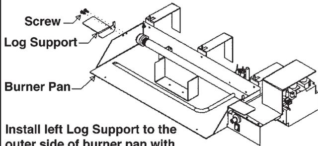
Install left Log Support to the outer side of burner pan with two 8-18 x DT Screws.
