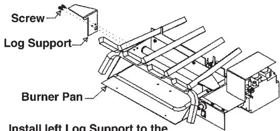
Install left Log Support to the outer side of burner pan with two 8-18 x DT Screws.
