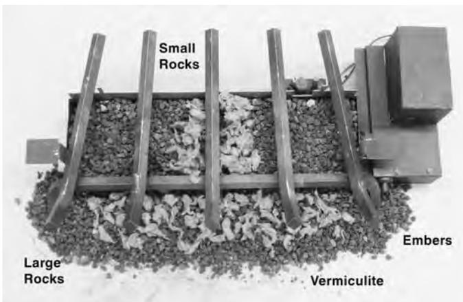
Place silica sand (NG only) or 1/4" small rock (LP only) inside and in front of burner pan. Place 1" large rock inside, in front, and around the sides of the pan. Place rock wool inside the middle of the pan and also in front of the grate bar. Sprinkle vermiculite over top of lava rock and rock wool.
