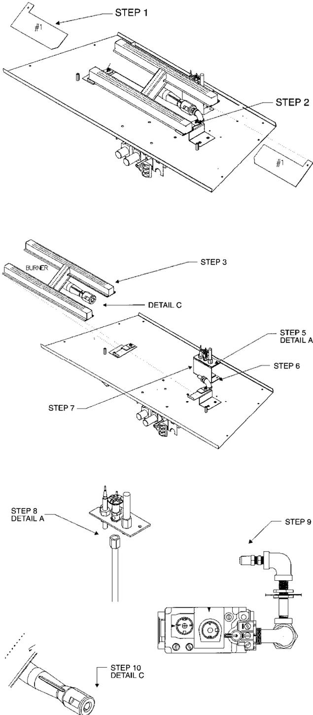
1. Remove the 2 ember plates from the burner. This step may not be required, depending on the type of burner assembly.
