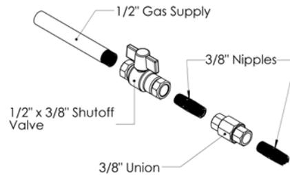
Important: Always check for gas leaks with a soap and water solution. Do not use open flame for leak testing.
