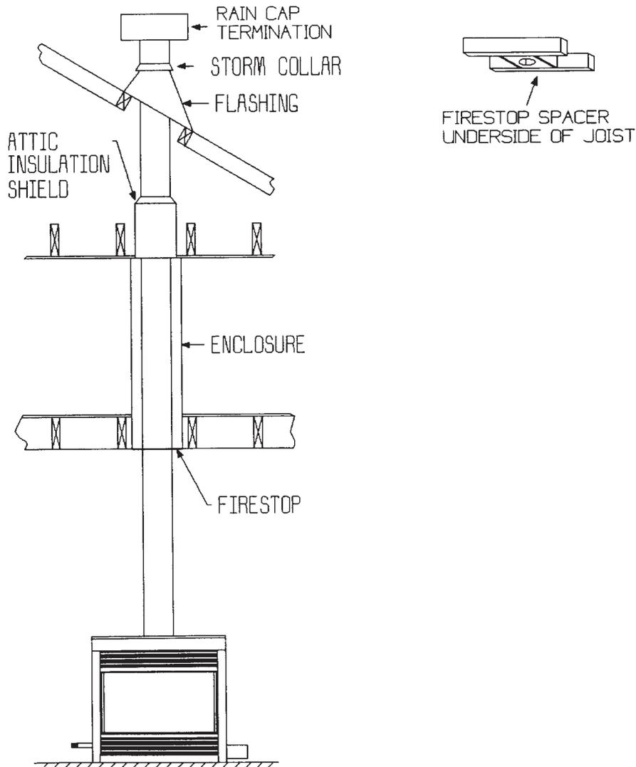
**A chimney venting this fireplace shall not vent any solid fuel burning appliance.**
