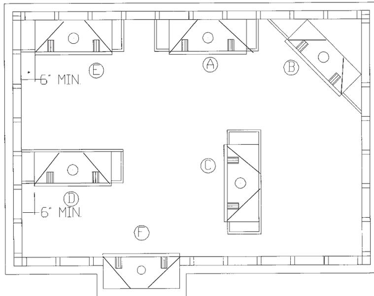
When you install your fireplace as in position 'B', 'D' or 'E', a minimum of 6 inches (153mm) clearance must be maintained from the perpendicular wall and the front of the appliance.
