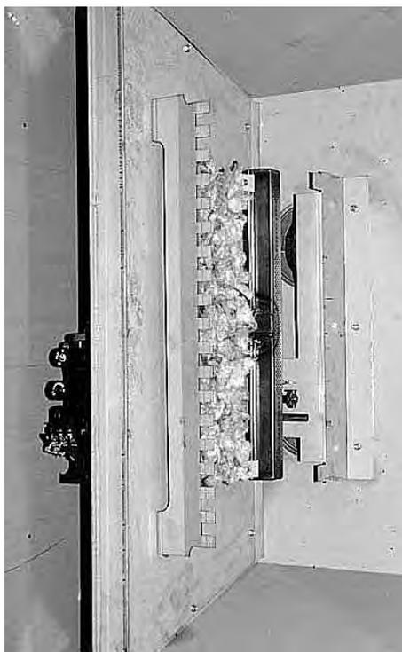
**Step (4)** Break glowing embers into thumbnail size. Place glowing embers on to the surface of the front burner, to the surface of the ember plates and over crossover to the same height as ember plates.
