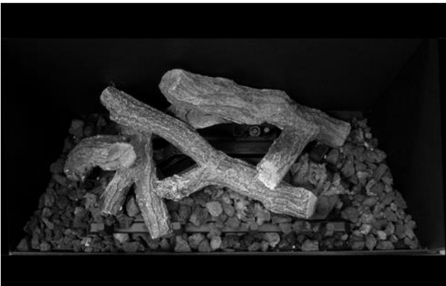
STEP 5: Fill in the rest of the burner pan and ember plates with lava rock and vermiculite. Do not place lava rock or vermiculite on any of the burner ports.
