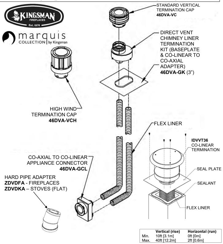
These kits may be used when installing a fireplace using a masonry chimney.
