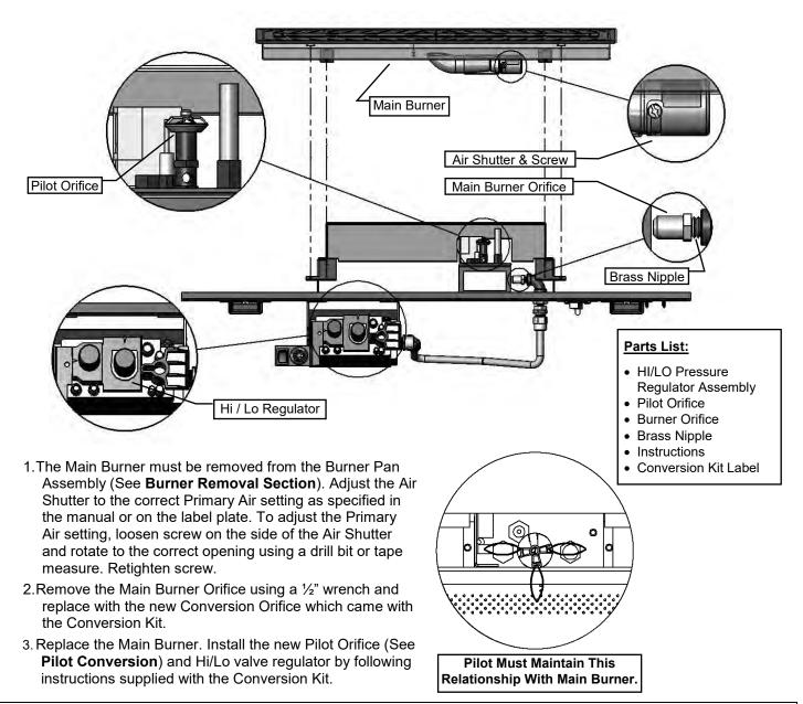
Refer to "Gas Specifications Chart" for inlet pressures and input ratings. Clock meter to verify input rate. Place conversion label as close to converted gas control as possible. Refer to lighting instructions to verify the normal operating sequence of the ignition system.
