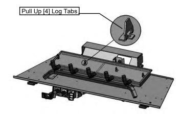
Pull up [4] Log Tabs on Burner. Match with Holes in Logs 3 & 4.
