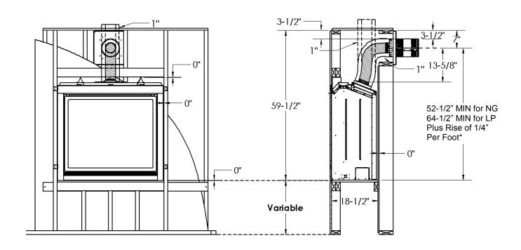
\*Note: If appliance is installed directly on carpeting or other combustible material other than wood flooring, a metal or wood panel extending the full width and depth of the appliance must be used. Carpet may extend 1 inch above the floor of the appliance.
