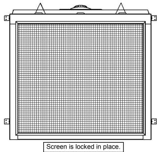
To remove Safety Screen, **WAIT UNTIL FIREPLACE IS COMPLETELY COOL.** Push up at center of Screen Frame and pull bottom away from fireplace.
