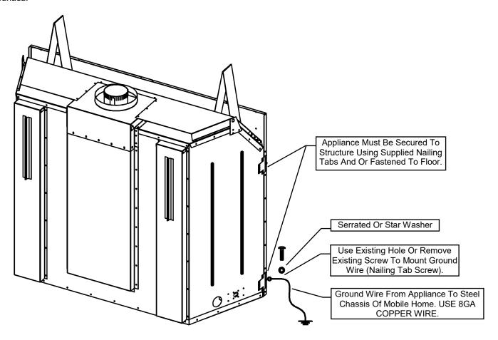
THE VENTED GAS FIREPLACE HEATERS IN THIS MANUAL MAY BE INSTALLED IN MANUFACTURED (MOBILE) HOMES AFTER FIRST SALE IN THE USA.
