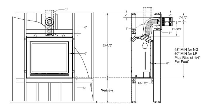
\*Note: If appliance is installed directly on carpeting or other combustible material other than wood flooring, a metal or wood panel extending the full width and depth of the appliance must be used. Carpet may extend 1 inch above the floor of the appliance.
