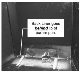
Step Two: Place Back Liner against back wall of firebox. NOTE: For Ceramic Glass units (ZCV39NH, ZCV39NEH, ZCV39LPH, ZCV39LPEH, ZCV42NH, ZCV42NEH, ZCV42LPH, and ZCV42LPEH) burner must be removed. See Burner Removal section of manual.
