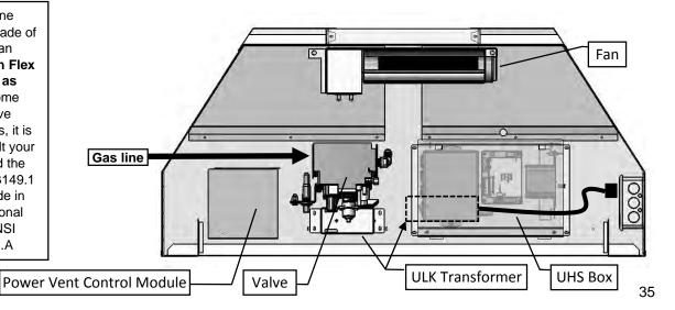
The fan can be installed through the side of the fireplace.
