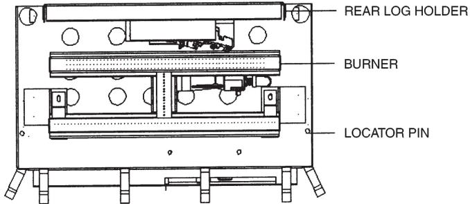
STEP 1 Locate hole on underside of log and place log over burner and Locator Pin and lower into position.
