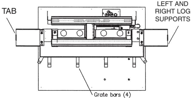
STEP #1. Locate Log #1 by positioning notches on under side of front log with the front Grate bars (4) and pull forward.
