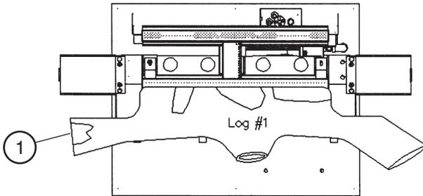
STEP #2. Locate left front Log by positioning slot on bottom of log with Tab on support bracket and lower into position.
