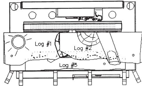
STEP 2 Locate hole on underside of log and place log over burner and Locator Pin and lower into position.
