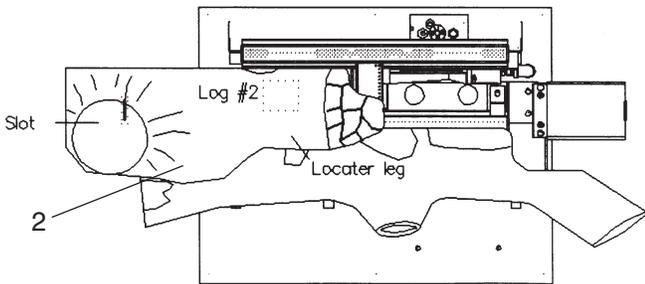
STEP #3. Locate right front Log by positioning slot on bottom of log with Tab on support bracket and lower into position.
