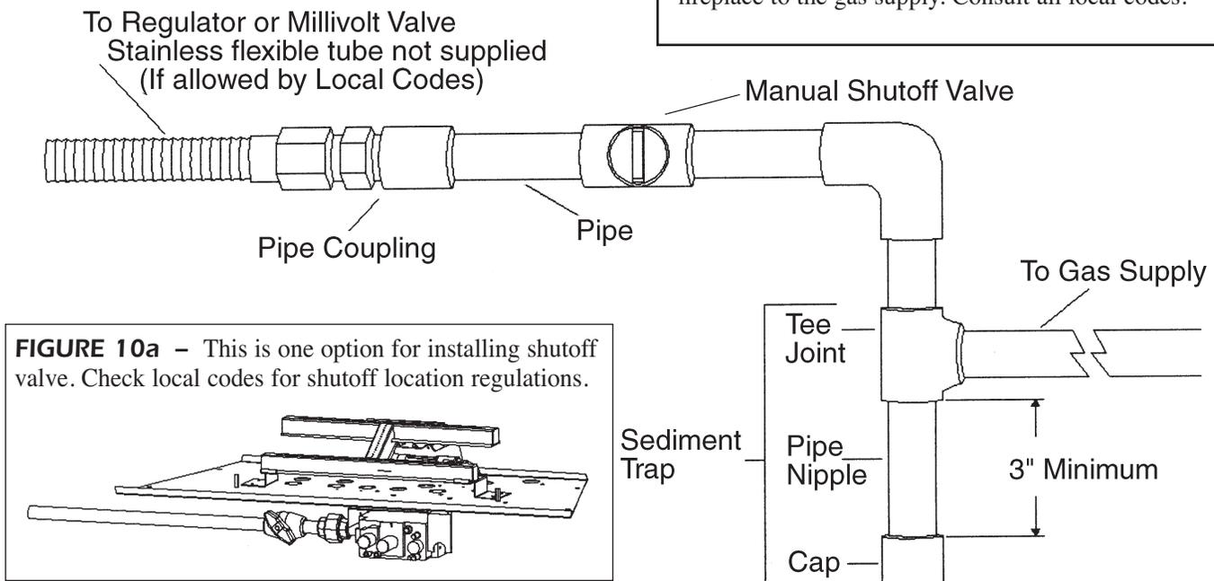
**FIGURE 10a** – This is one option for installing shutoff valve. Check local codes for shutoff location regulations.
