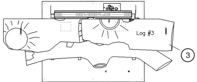
STEP #4. Place rear log onto rear log holder and pull up to left and right front logs.
