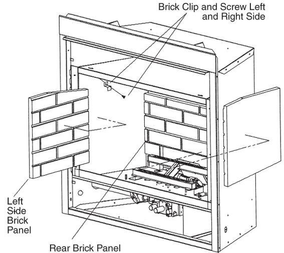
FIGURE 13 – Installing Brick Panels
