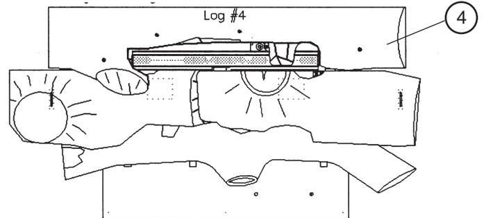
STEP #5 & 6. Line up holes on crossover logs with locator pins on rear log #4 and lower into position.
