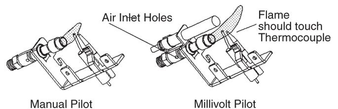
FIGURE 11 – Manual and Millivolt Pilot Flames
