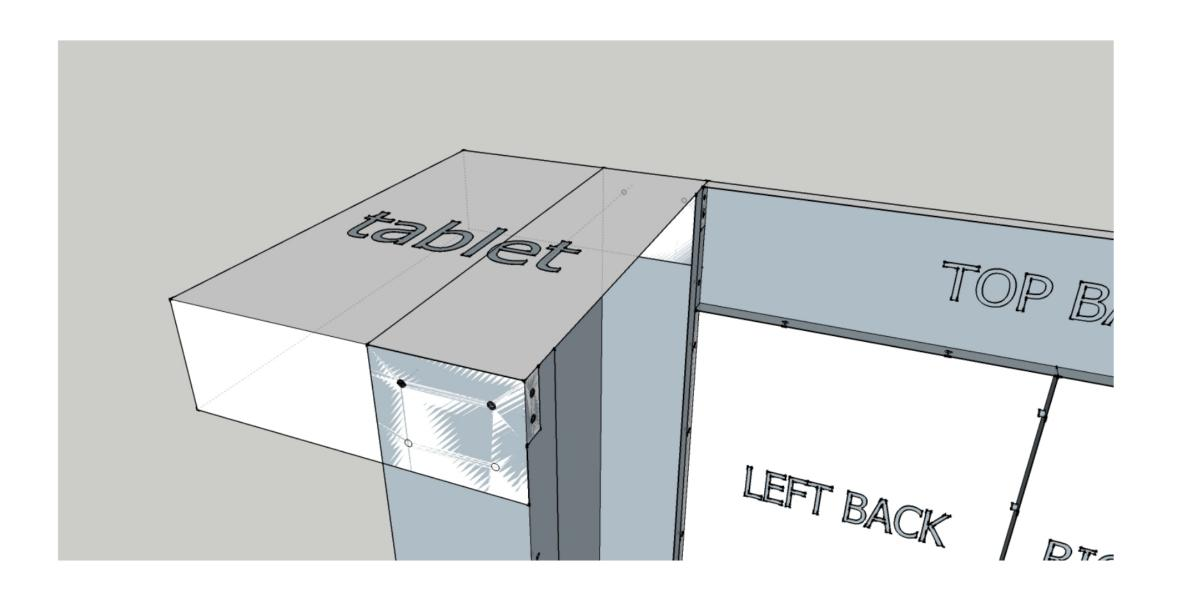
8-2 TABLET: Add the right tablet, fix it with 10 M4 screws
