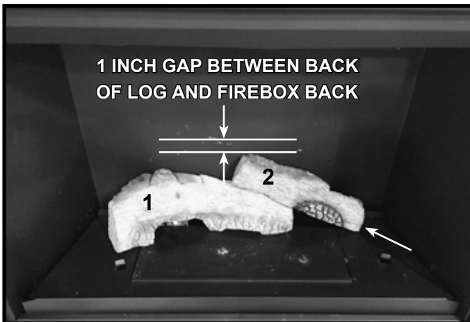
Figure 5. Install Right Rear Base Log
