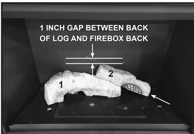
Figure 5. Install Right Rear Base Log
