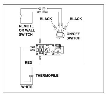
Figure 3. Standing Pilot Wiring Diagram
