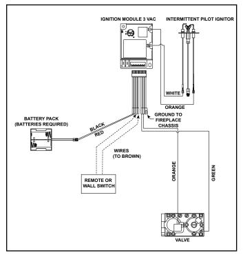
Figure 2. IPI Wiring Diagram-CFL-24NG-IPI and CFL-24LP-IPI
