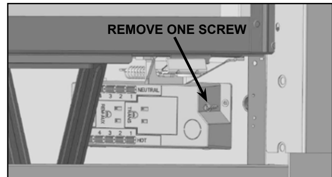
Figure 8.3 Junction Box Detail - JADE32IN
