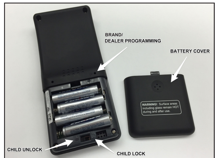
Figure 1. Install Batteries & Child Safety
