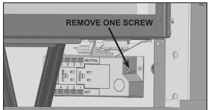
Figure 8.3 Junction Box Detail - JADE32IN-B
