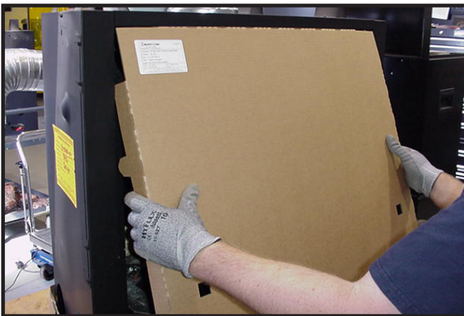
Figure 11.5 Installation of Splatter Guard
