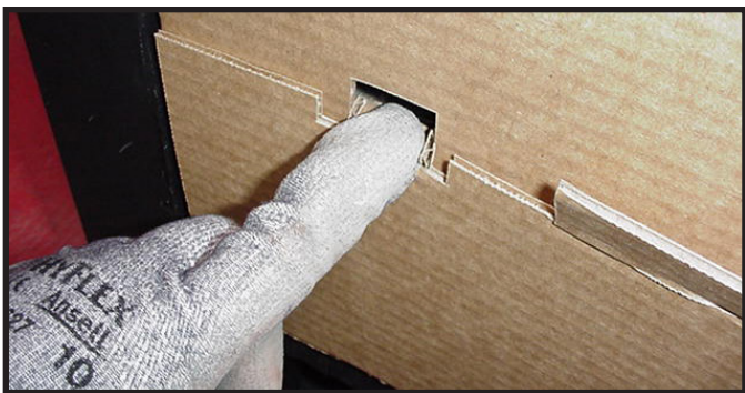
Figure 11.10 Securing Tabs Inside Front of Splatter Guard
