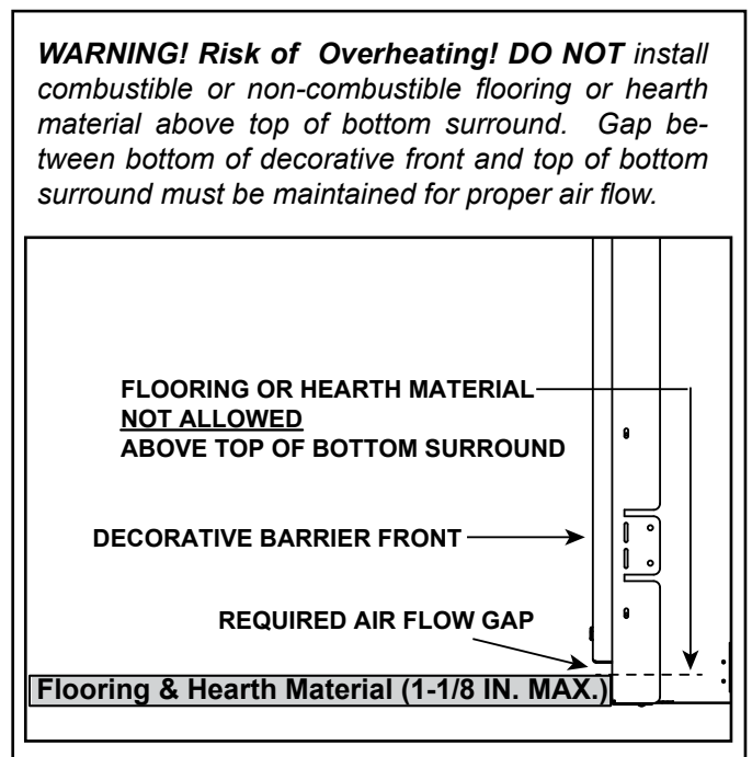
Figure 10.3 Required Air Flow Gap
