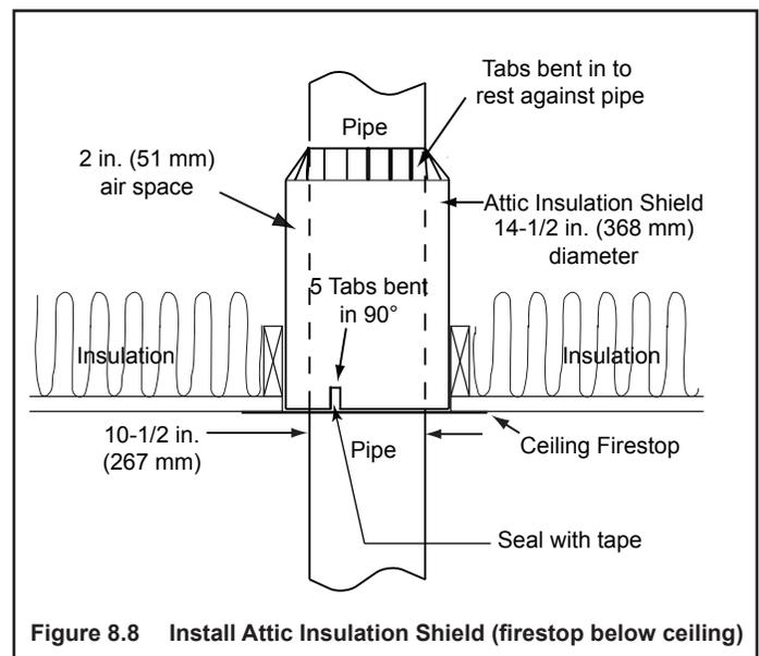
Figure 8.8 Install Attic Insulation Shield (firestop below ceiling)
