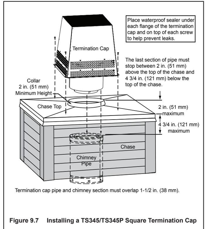
Figure 9.7 Installing a TS345/TS345P Square Termination Cap
