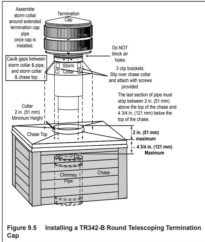
Figure 9.5 Installing a TR342-B Round Telescoping Termination Cap
