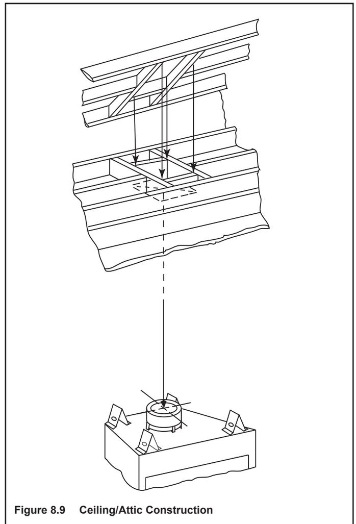
Figure 8.9 Ceiling/Attic Construction
