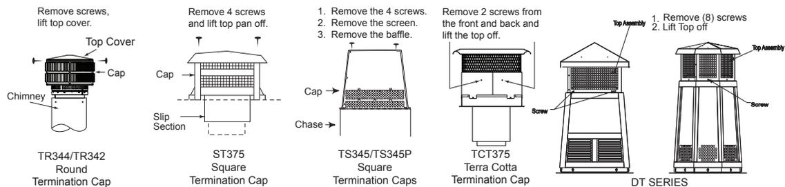
Figure 3.1 Chimney & Termination Cap Cleaning
