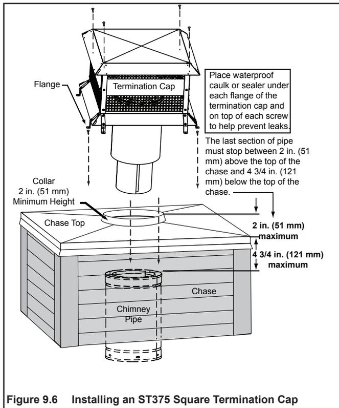
Figure 9.6 Installing an ST375 Square Termination Cap
