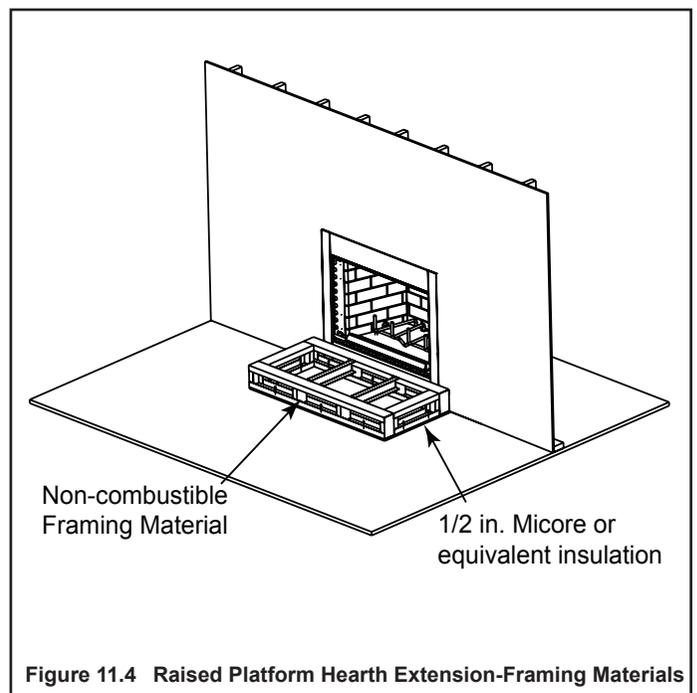
Figure 11.4 Raised Platform Hearth Extension-Framing Materials
