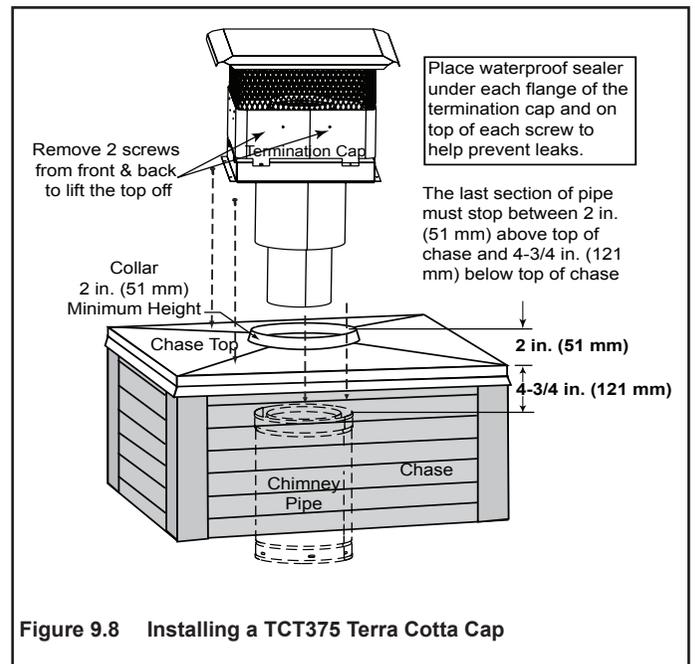
Figure 9.8 Installing a TCT375 Terra Cotta Cap
