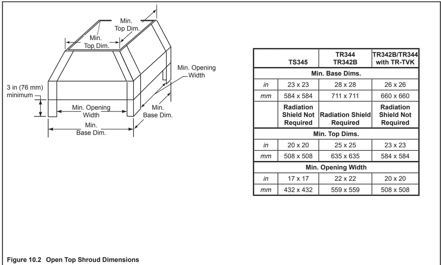
Figure 10.2 Open Top Shroud Dimensions
