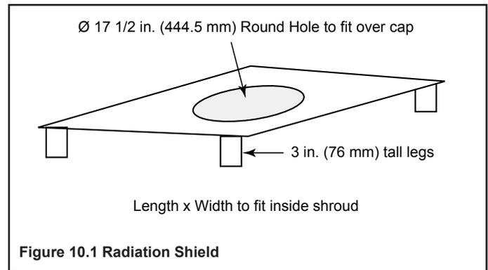
Figure 10.1 Radiation Shield
