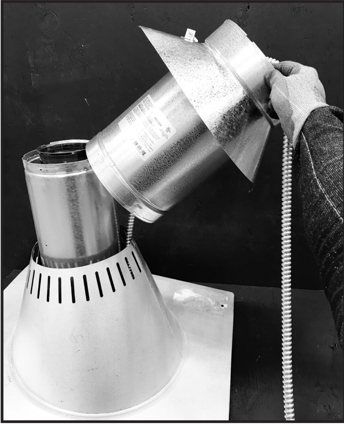
Figure 3.19 Route PVI Harness Through Flashing
