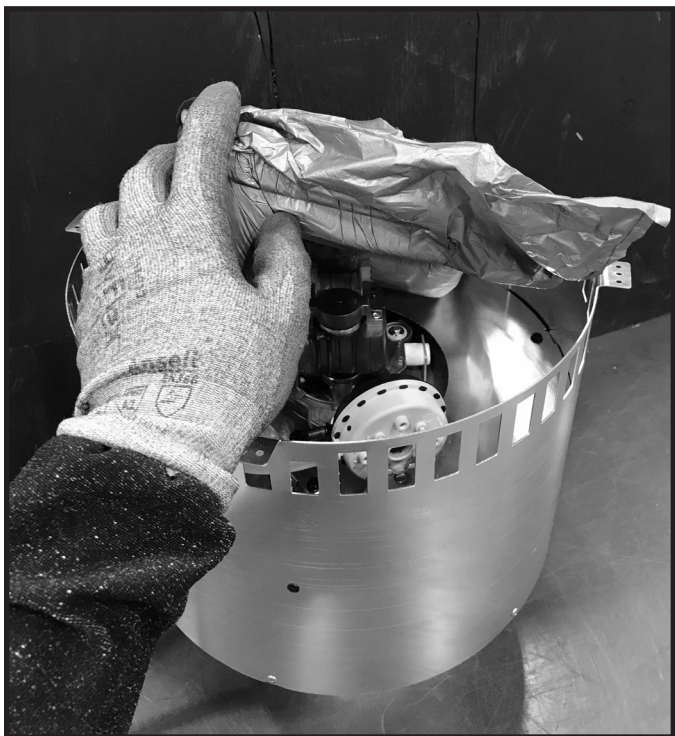
Figure 3.7 Remove Shipping Support Foam
