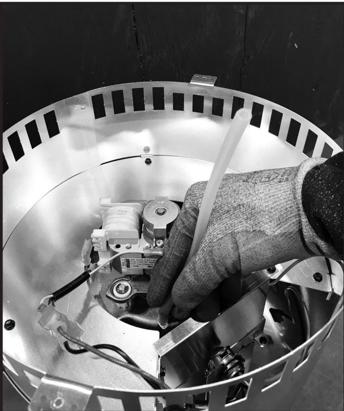
Figure 5.5 Remove Teflon Tubing from Blower
