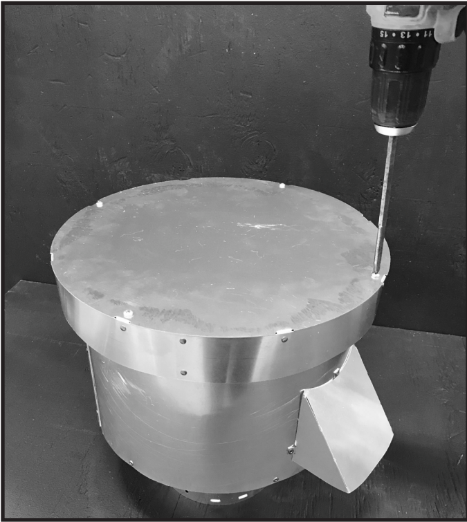
Figure 3.6 Remove Top Cap Screws
