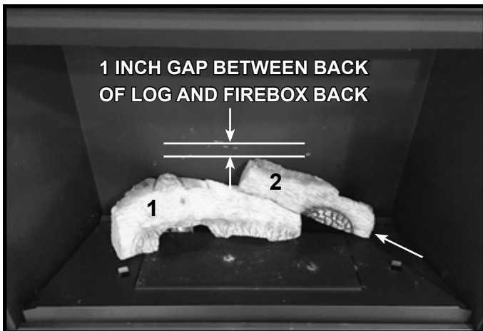
Figure 5. Install Right Rear Base Log
