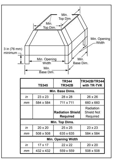
TR342 caps require radiation shield unless installed partially above the shroud. The TR cap must be raised to the minimum dimensions (or greater) above the shroud. Refer to Figure 6.3.
