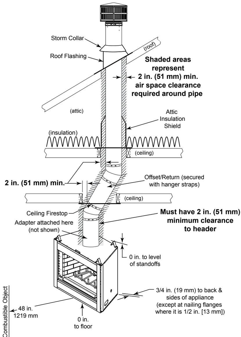
Figure 3.2 Clearances to Combustible Materials
