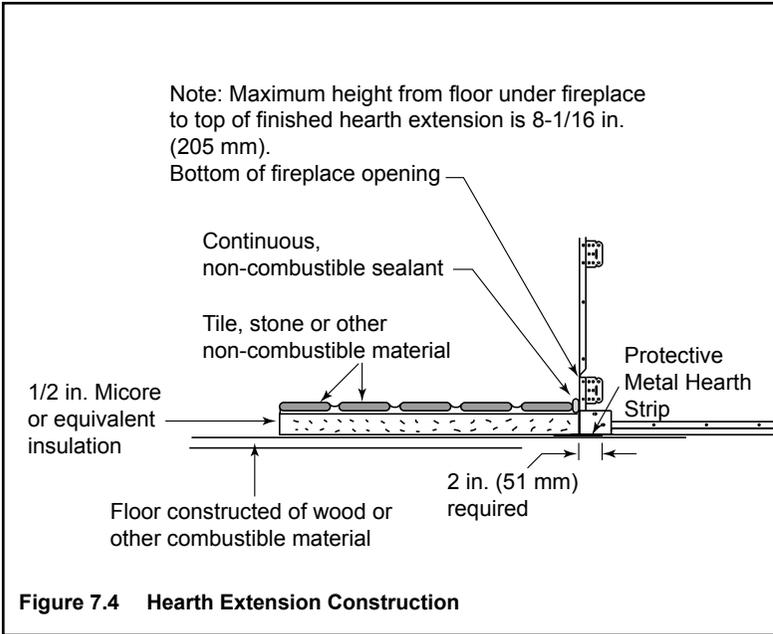
Figure 7.4 Hearth Extension Construction
