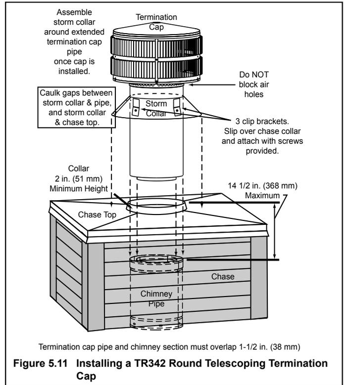
**Figure 5.11** Installing a TR342 Round Telescoping Termination Cap
