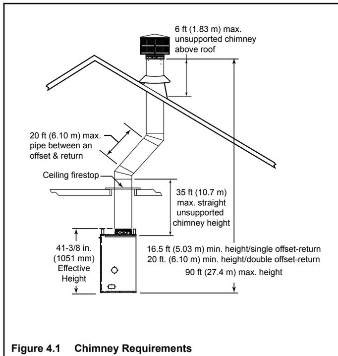
**Figure 4.1 Chimney Requirements**
