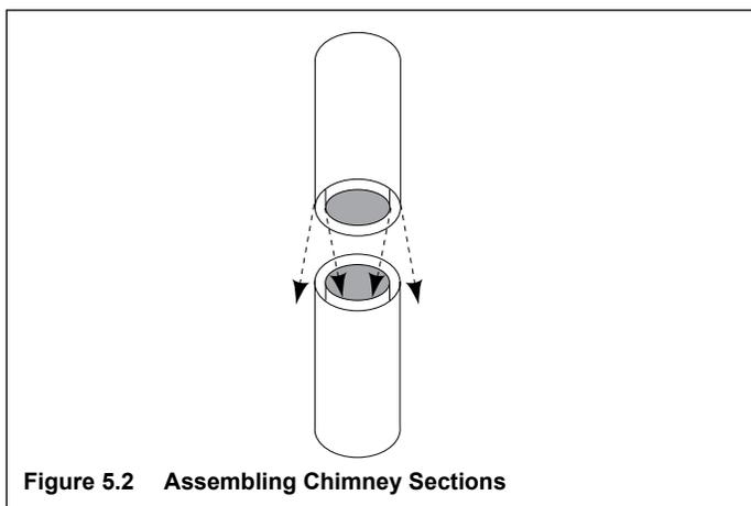
Figure 5.2 Assembling Chimney Sections
