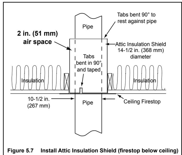
Figure 5.7 Install Attic Insulation Shield (firestop below ceiling)
