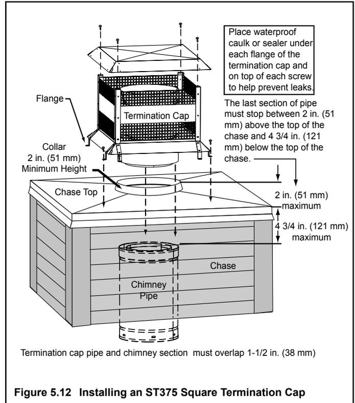
**Figure 5.12** Installing an ST375 Square Termination Cap
