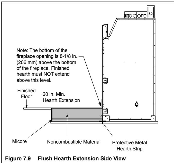
Figure 7.9 Flush Hearth Extension Side View
