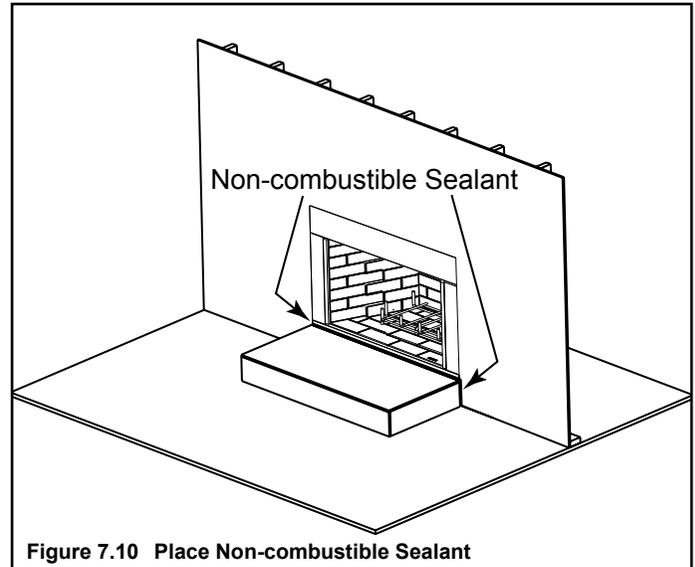
Figure 7.10 Place Non-combustible Sealant
