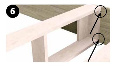
Continue to make sure shelf pins are secure and below each framing box for alignment and correct position.
