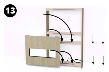
Mount fireplace front facia, by sliding onto attached upper and lower horizontal mounting strips secured to wall unit.
