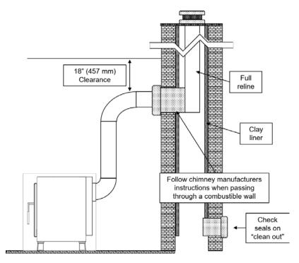
Special care must be taken regarding the wall thimble, or penetration from the chimney connector pipe to the masonry chimney, if the wall thimble must pass through an exterior wall. Here all chimney manufacturer's instructions must be followed, including guidance on spacing to combustible surfaces, piping requirements, and liner requirements. Check with local authorities before installation to ensure all requirement are met.
