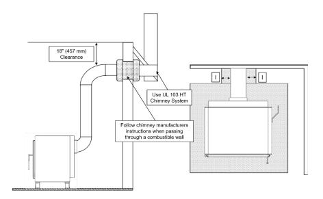
Minimum Clearance RequirementsI Floor protection, connector side2" (51 mm)
