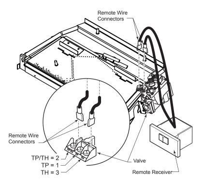
Figure 5.2 - Installing Remote Receiver
