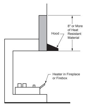
Figure 3.3 - Measuring Heat Resistant Material for Mantel
