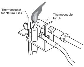
Figure 12.2 Incorrect Pilot Flame Appearance
