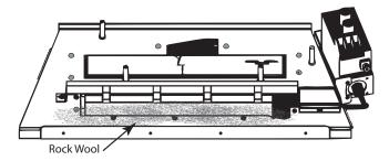
Figure 6.1 - Installing Rock Wool
