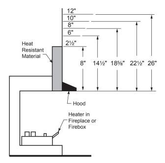
Figure 3.5 - Minimum Mantel Clearance with Hood — All Models
