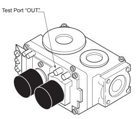
Figure 4.2 - Pressure Test Point Location Millivolt Control
