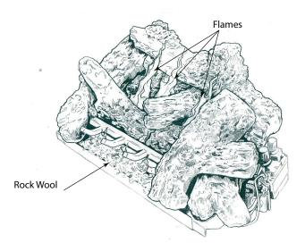
Figure 6.29 - Correct Appearance of Rear Flames
