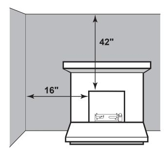
Figure 3.1 - Sidewall and Ceiling Clearances
