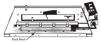
Figure 6.10 - Installing Rock Wool
