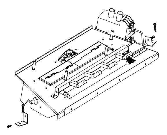
Figure 3.10 - Securing Heater to Floor of Fireplace/Firebox
