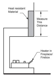
Figure 3.2 - Measure Heat Resistant Material
