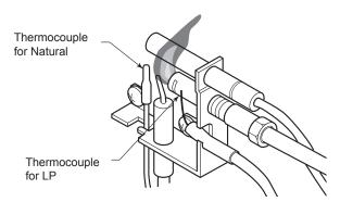
Figure 6.28 - Incorrect Appearance of Pilot Flame
