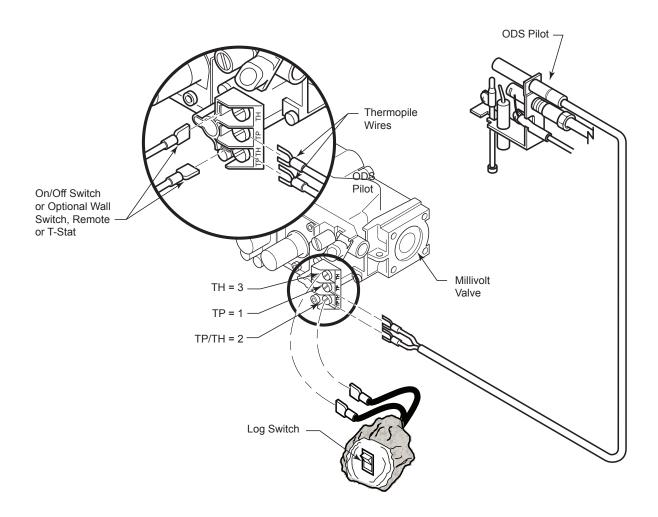
Figure 5.1 - Wiring Diagram NOTE: Log switch wires are not factory connected. Connect log switch wires to the TP/TH and TH valve terminals as shown.
