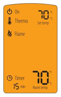
Figure 9. RC300 Idle Mode
