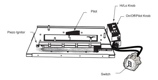
Figure 10.1 - Location of Piezo Ignitor, Control Knobs and Switch
