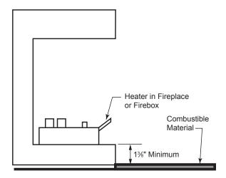
Figure 3.7 - Minimum Clearance above Combustible Flooring
