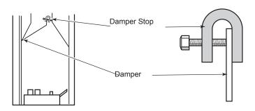
Figure 3.9 - Damper Stop Installation.
