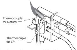
Figure 6.27 - Correct Appearance of Pilot Flame
