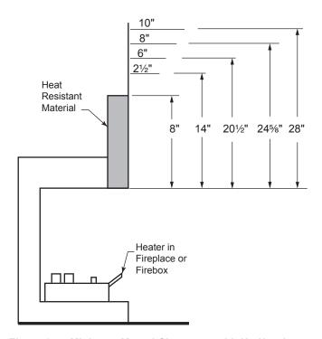
Figure 3.4 - Minimum Mantel Clearance with No Hood — GG18
