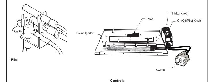
Figure 10.2 - Piezo Ignitor
