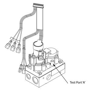
Figure 4.3 Pressure Test Point Location
