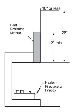
Figure 3.6 -Minimum Mantel Clearance with No Hood — GG18/24
