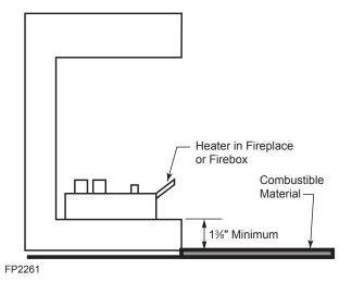
Figure 11 Minimum Clearance above Combustible Flooring
