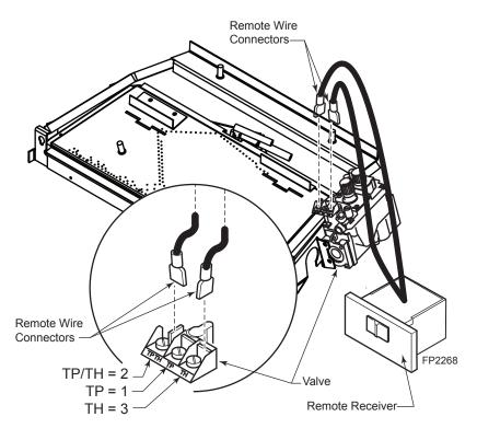
Figure 18 -Installing Remote Receiver
