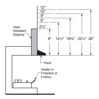
Figure 8 - Minimum Mantel Clearance with Hood — All Models
