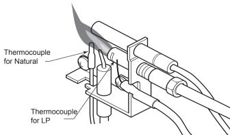
Figure 49-Correct Appearance of Pilot Flame
