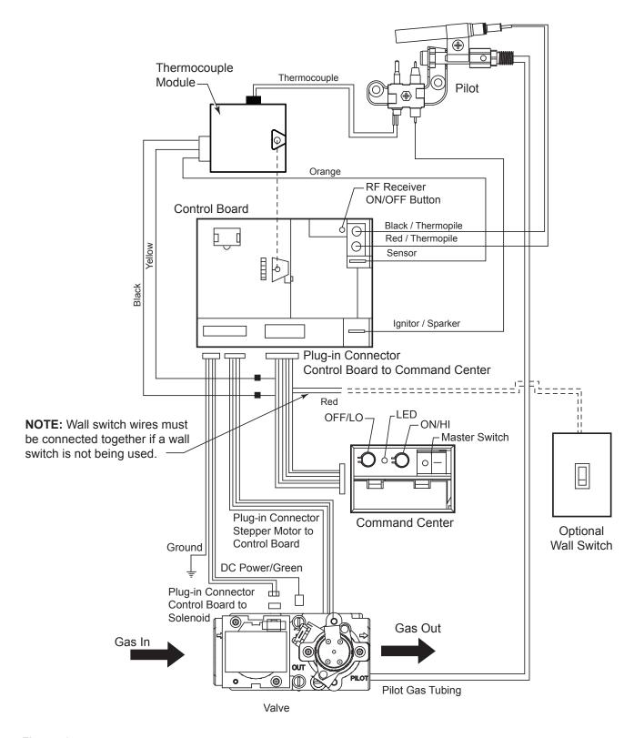
Figure 53 -Signature Command Wiring Diagram
