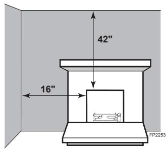
Figure 4 - Sidewall and Ceiling Clearances
