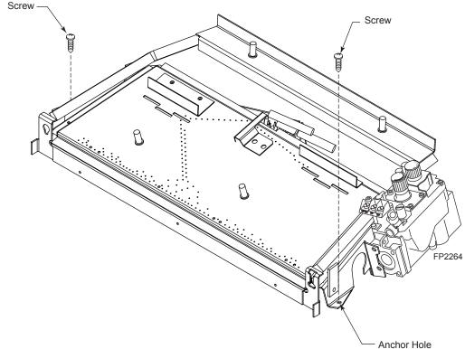
Figure 14 - Securing Heater to Floor of Fireplace/Firebox
