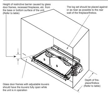
Figure 2 Reference Drawing of a Natural Flame Log Set in an Enclosure
