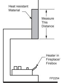
Figure 5 - Measure Heat Resistant Material
