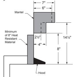
Figure 10 - Minimum Mantel Clearance with Hood — NB24 (Example of Unsafe Installation)
