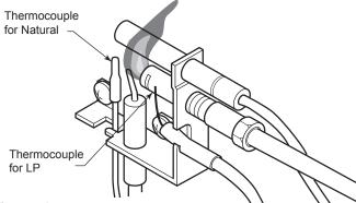
Figure 50 - Incorrect Appearance of Pilot Flame
