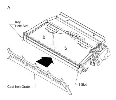
Figure 19 -Install Cast Iron Grate
