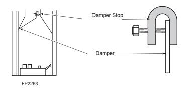
Figure 13 - Damper Stop Installation.
