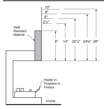
Figure 7 Minimum Mantel Clearance with No Hood — NB18
