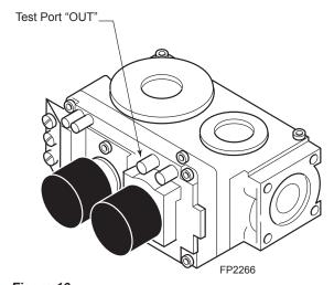
Figure 16 -Pressure Test Point Location Millivolt Control
