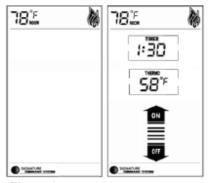
2. B) Mode. The transmitter always displays all available icons showing current status of timer and thermostat as shown in the figure on the right.
