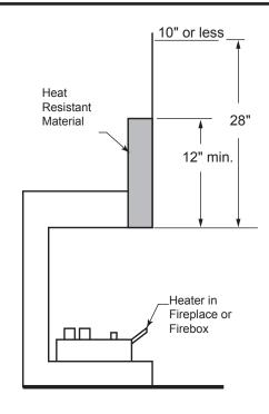
Figure 9 - Minimum Mantel Clearance with No Hood — NB24
