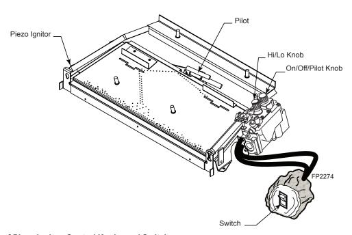
Location of Piezo Ignitor, Control Knobs and Switch
