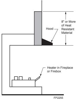
Figure 6 - Measuring Heat Resistant Material for Mantel
