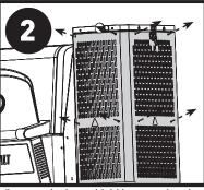
Remove the heat shield by removing the top and bottom screws.
