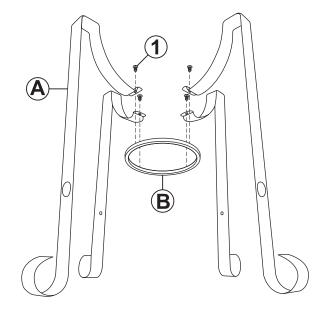
Align the holes in Small Ring (B) with the bottom of four Legs (A), as shown. Loosely attach the ring to the legs by hand-tightening four M6x8mm Bolts (1).
