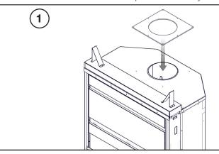
Install the 10" anchor plate gasket concentric to the flue collar.
