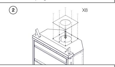
Install the anchor plate with 8 screws (provided) concentric to the flue collar.
