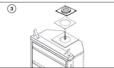
Install the 8" gasket and your chimney supplier's insulated chimney anchor plate.
