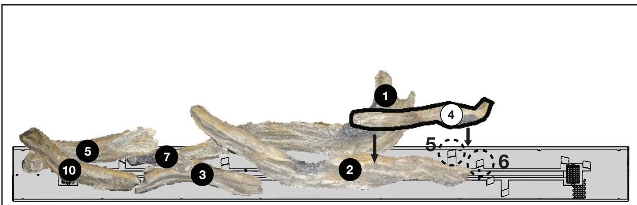
7. With the charred end on the media tray, place Log #4 between tabs #5 & 6. Rest the opposite end in the locating groove of Log #2.
