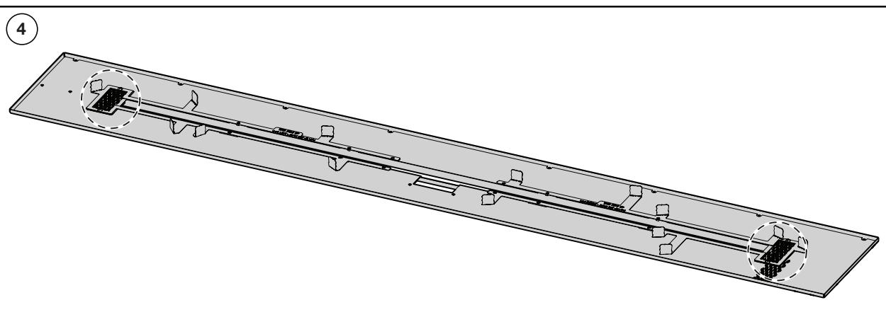
Ensure the mesh covers are secured back in place.
