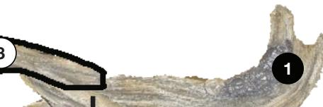
3. With the charred end facing the burner, place Log #3 in front of locating tabs #10 & 11. Ensure the log is against the tabs.
