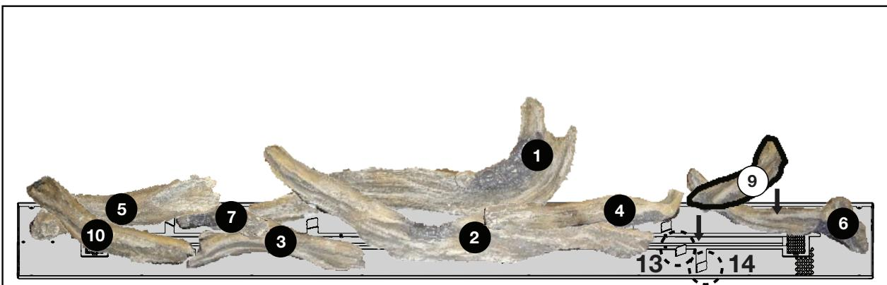
9. Place the pointed end of Log #9 between locating tabs #13 & 14 and rest the opposite end on Log #6. Ensure the charred side is facing the burner.
