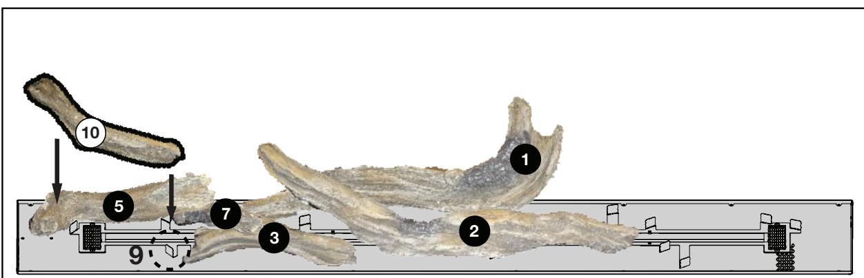
6. With the charred side facing the burner, place the pointed end of Log #10 on the media tray in front of tab #9. Ensure the log is against the tab. Rest the opposite end on Log #5.
