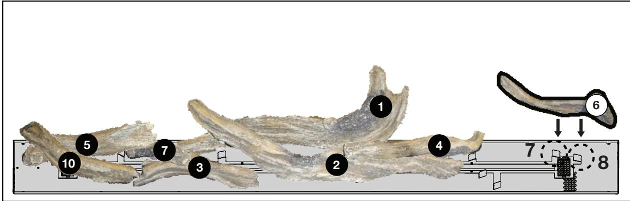
8. Place Log #6 in front of locating tabs #7 & 8. Ensure the log is against the tabs.
