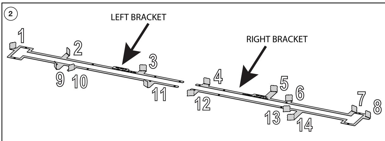
Once apart, using a pair of pliers bend the 10 locating tabs to 90°.
