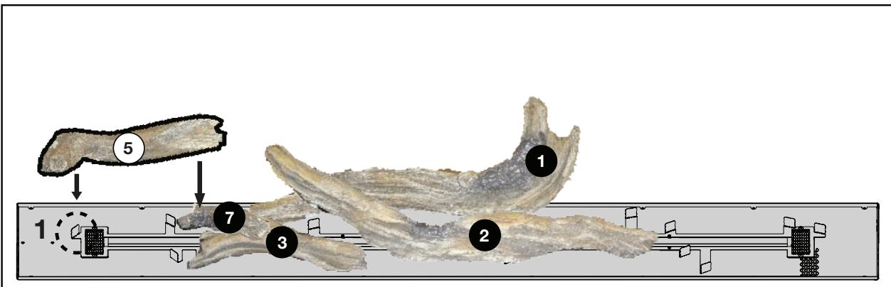
5. Place the curved end of Log #5 on the media tray behind locating tab #1. Rest the opposite end on top of Log #7.
