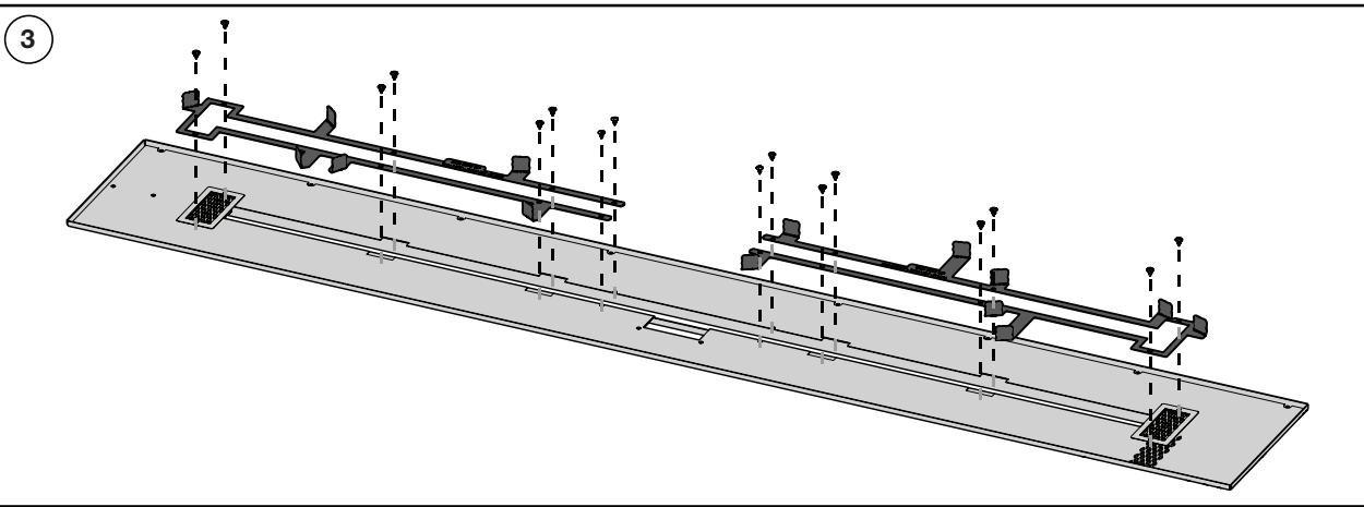
Starting on the left side of the unit. Remove the 8 screws from the media tray and burner. Place the left bracket on top of the media tray and burner securing it with the screws just removed. Repeat the process for the right side.
