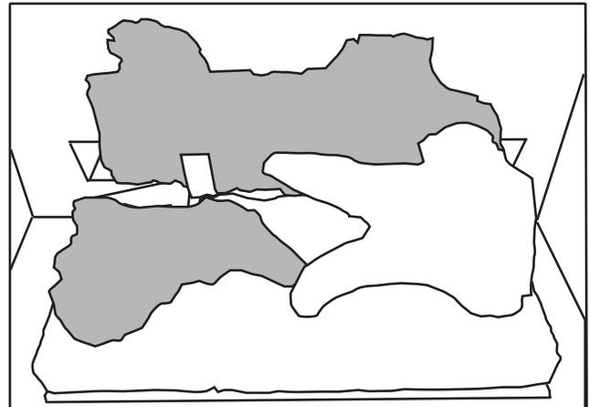
**C.** Place the hole in the underside of log #3 onto the locating screw, on the right side of the burner. The bottom branch of log #3 sits in front of, and against, the right end of log #2.
