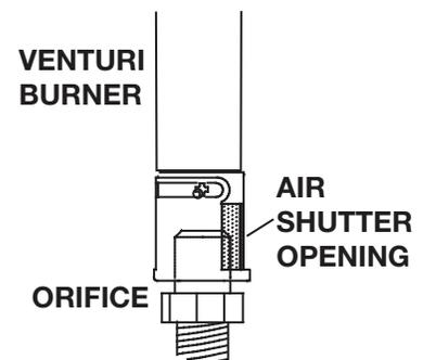
Remove the 2 screws securing the burner. Air shutters have been factory set open according to the Venturi Adjustment Chart. These settings are for (maximum) horizontal termination. Adjustment may be required depending on fuel type, vent configuration and altitude. After making adjustments replace the burner ensuring that the venturi tube fits over the orifice and replace the screws.
