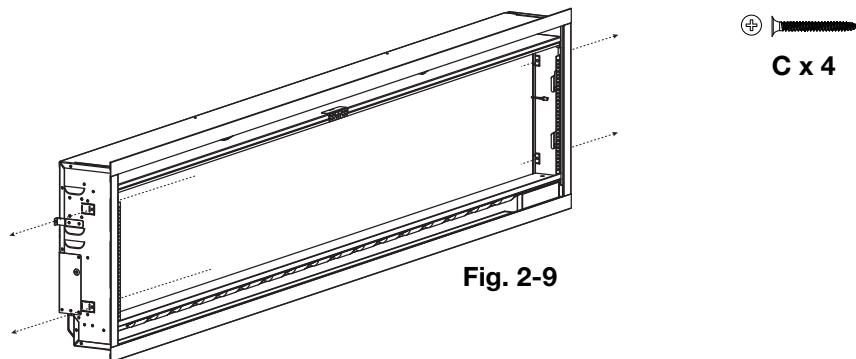
10. Reinstall the plastic panel holding bracket.
