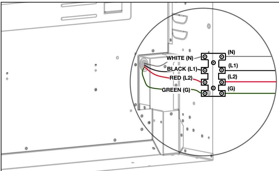
1. Remove the securing screws from the junction box cover plate, located on the left side, at the back of the appliance. Discard the original junction box cover plate and set screws aside.
