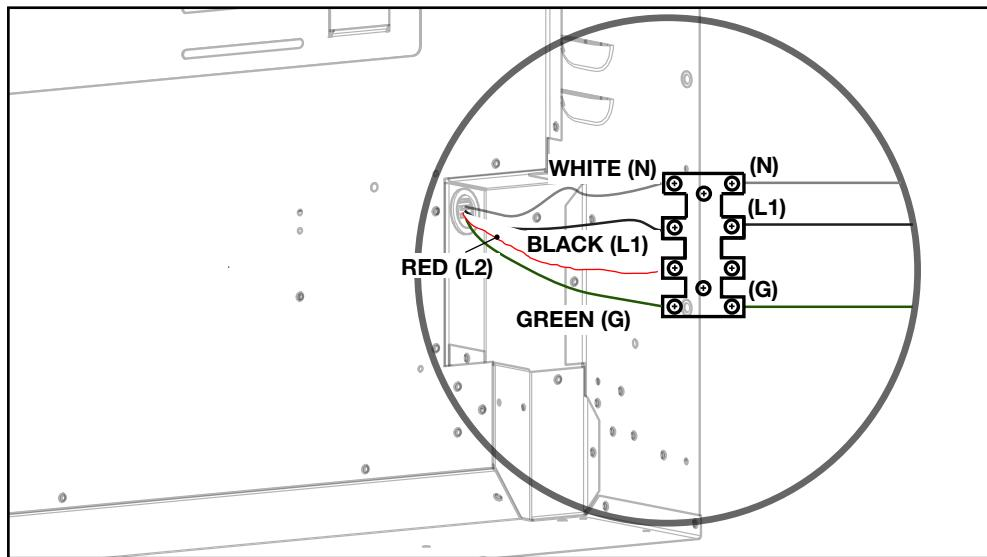
1. Remove the securing screws from the junction box cover plate, located on the left side, at the back of the appliance. Discard the original junction box cover plate and set screws aside.
