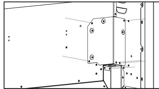
Before hardwiring the appliance, remove the junction box control cover by removing the fasteners as shown.
