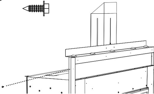
Secure to the upper front frame using 2 screws (supplied).
