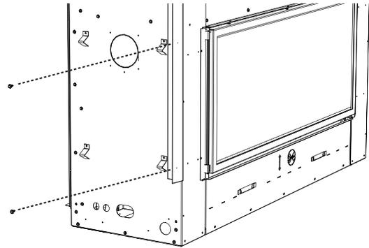
Align the nailing tab with the holes on the appliance, secure with the screws in step 1.
