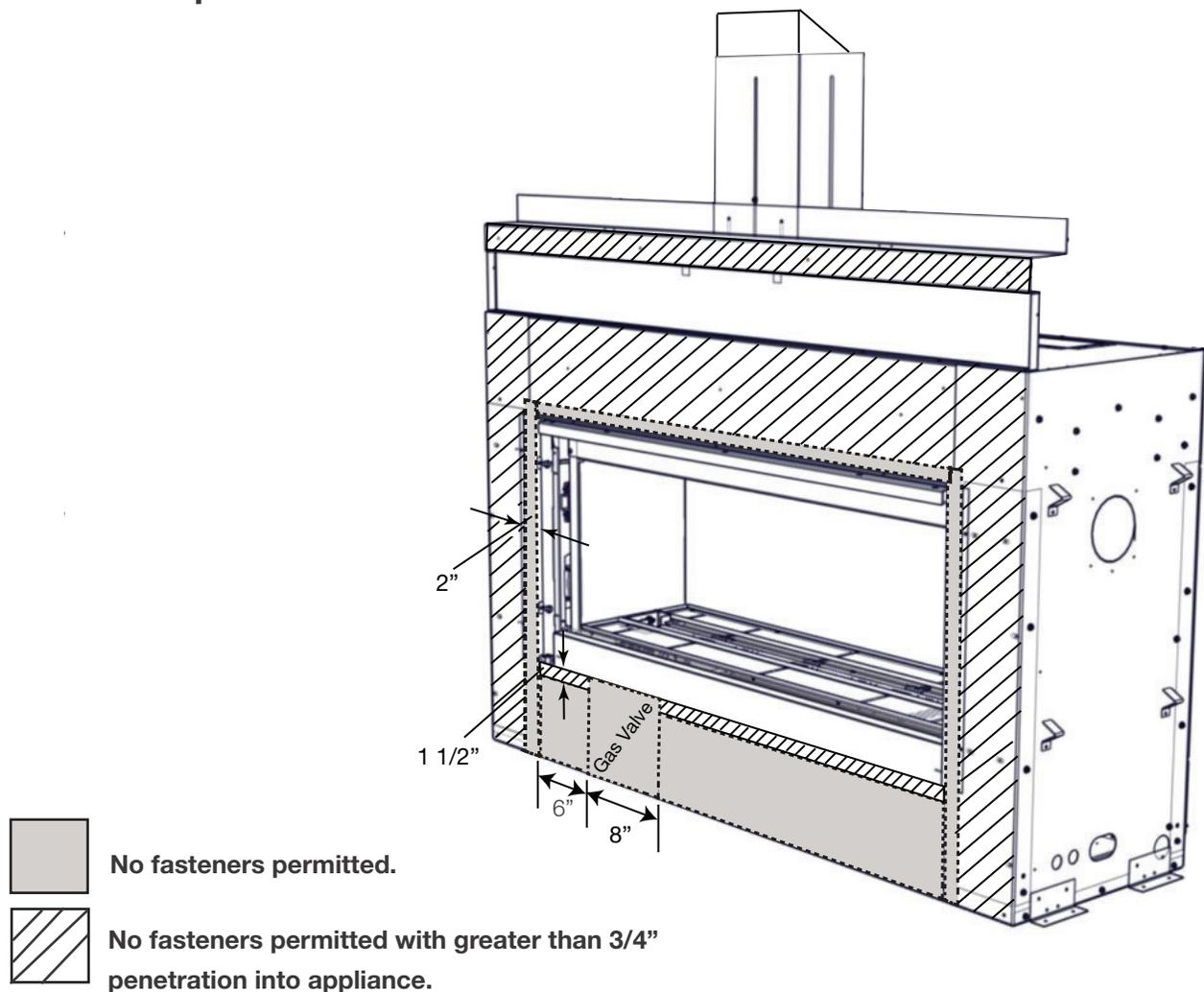
When securing non-combustibles, we suggest using high temperature construction adhesive within 2" (5.08cm) above and to the sides from the appliance opening and 8" (20.3cm) below the appliance opening. **DO NOT SCREW IN THE RESTRICTED AREA AS THIS COULD DAMAGE THE INTERNAL COMPONENTS OF THE APPLIANCE THAT CAN CAUSE INJURY OR DEATH.**
