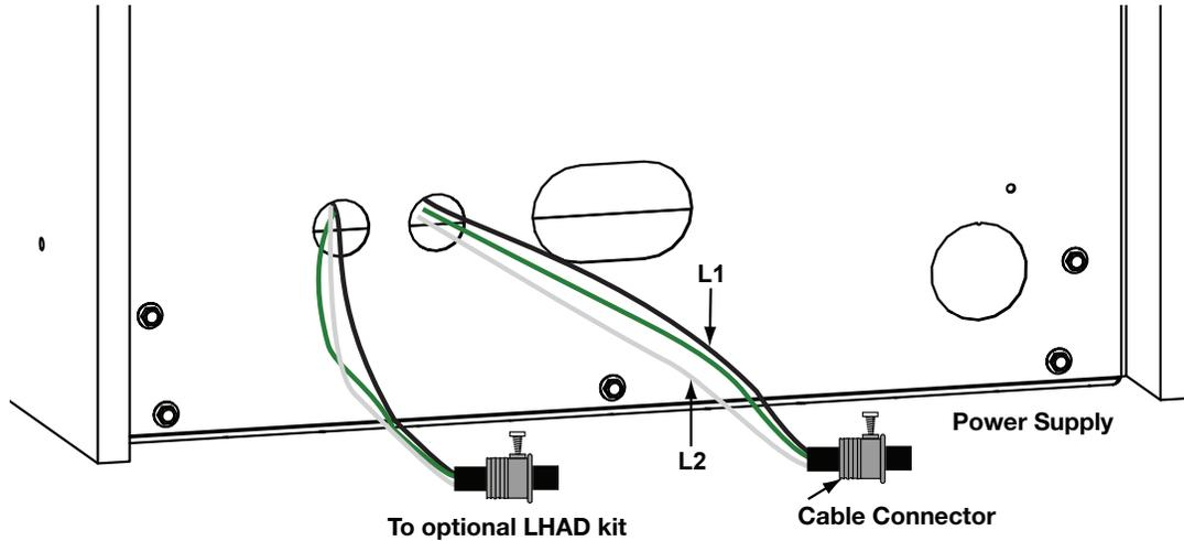
Route power supply and optional LHAD kit through the outer firebox to the receptacle mounted on the bottom of the appliance. For optional LHAD kit installation, please refer to the leaflet provided in the kit.
