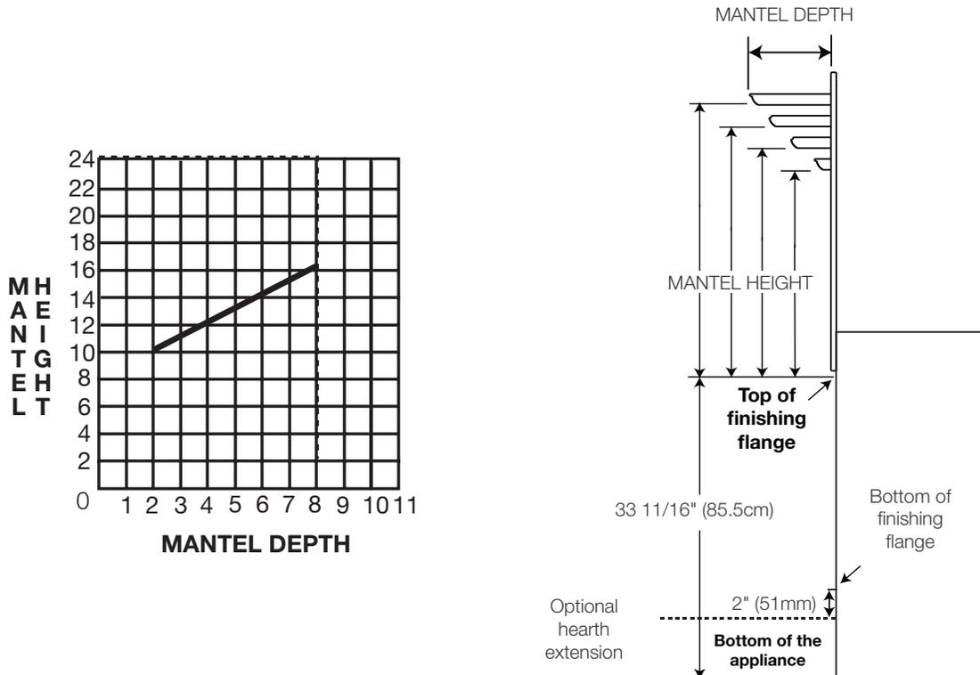
Installing a mantel between this appliance and electronics or other materials that may be sensitive to heat, will reduce the effect of direct heat on them. Ensure mantel is properly sized (width & depth) to suit the object being mounted above.
