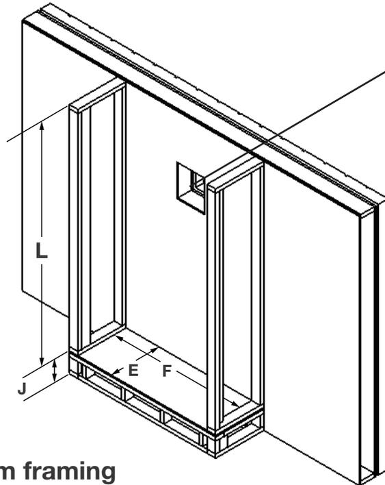
Before framing an appliance, ensure to install the firestop first.
