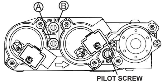
**After taking pressure readings, be sure to turn screws clockwise firmly to reseal. Do not overtorque.**
