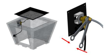
Attach flex line from the burner to gas valve as shown.
