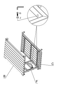
**3.** Using 4X M6\*30 Bolts (**G**) and 4X M6\* $\emptyset$ 16 Washers (**J**), attach Back Panel (**D**) to both Side Panels (**B & C**) as shown in image below. Loosely tighten with supplied allen wrench.
