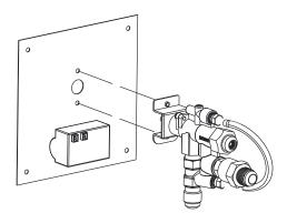
• For hard piped installations. Connect the gas supply line (not included) to the 3/8" male flare fitting on the valve. USE TWO WRENCHES TO ENSURE A GAS TIGHT CONNECTION.
