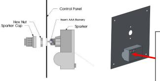
Located and orient sparker box on control panel as shown. Sparker box must be installed **before** burner valve.
