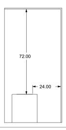
Burner model shown may not be the same model as your burner. Clearance requirement is 72" from top of burner to any overhead combustible materials and 24" from edge of burner trim to any combustible side walls. Burner Inserts (BI models) must follow the clearances for their corresponding CFP model.
