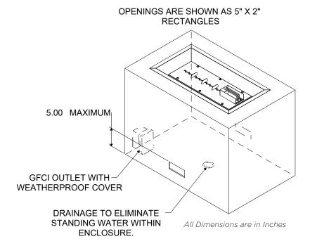
A readily accessible GFCI outlet should be installed within the enclosure to local electrical code. A weatherproof cover should be used. If outlet will not be readily
