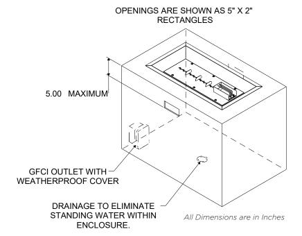
A readily accessible GFCI outlet should be installed within the enclosure to local electrical code. A weatherproof cover should be used.
