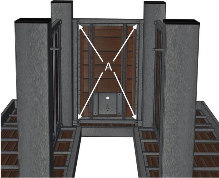
6. Attach **Center Support**, as shown below, to the bottom of the fire pit using **Bolt A (4X)**.
