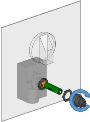
CF-SPARKER will not operate correctly without an ignition **and** ground wire attached.
