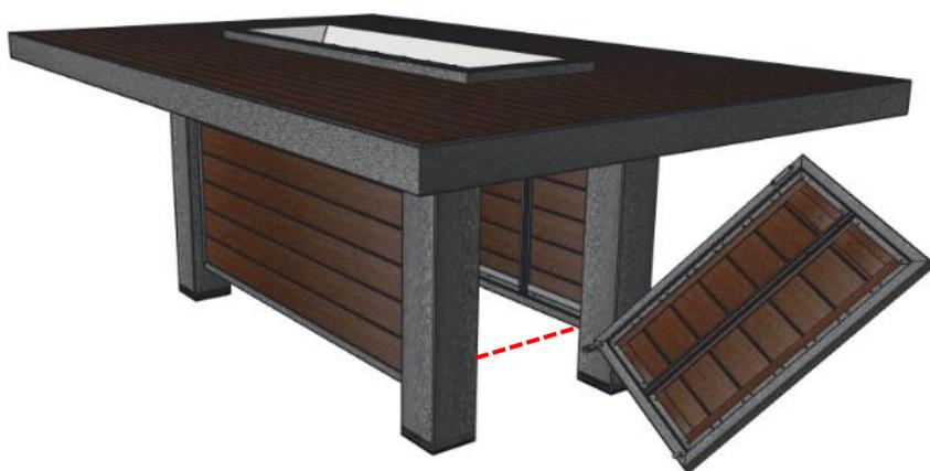
1. Connect the propane hose/regulator to the propane tank and hand tighten (**DO NOT USE A WRENCH**) and slide the propane tank past the dotted line to ensure the **Access Door** closes properly. Attach the **Access Door**.
