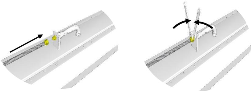
3. Set Burner into the fire pit base as shown below.
