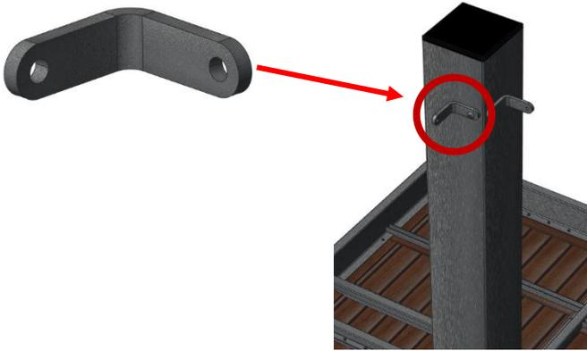
4. Attach **Panel A** using **Bolt A (4X)** to legs as shown below. Attach bottom of panel first with the help of the side support brackets. Next attach top of panel to upper support brackets. Repeat process for opposite side.
