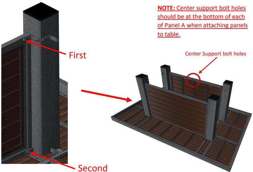
5. Attach **Panel B** using **Bolt A (4X)** as shown below.
