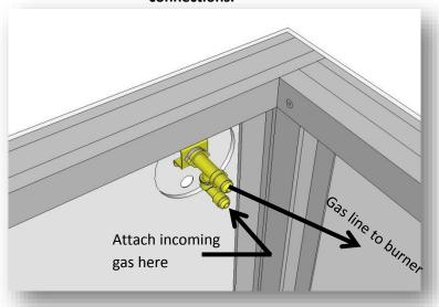
Do not make gas connections to burner until concrete, tile, or granite top is installed. Gas connections can be made from below or from above by lifting burner out of top to access gas line.
