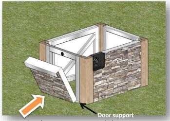
Set door on supports and close. Magnet will hold door in closed position.
