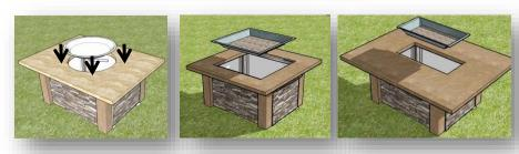
Lower burner onto base with burner neck facing in the direction of control panel location.
