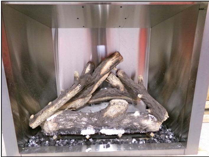
7. After the logs are installed place the lava rock/charcoal provided around the logs on the floor of the firebox. Ensure lava rock/charcoal does not cover any burner ports.
