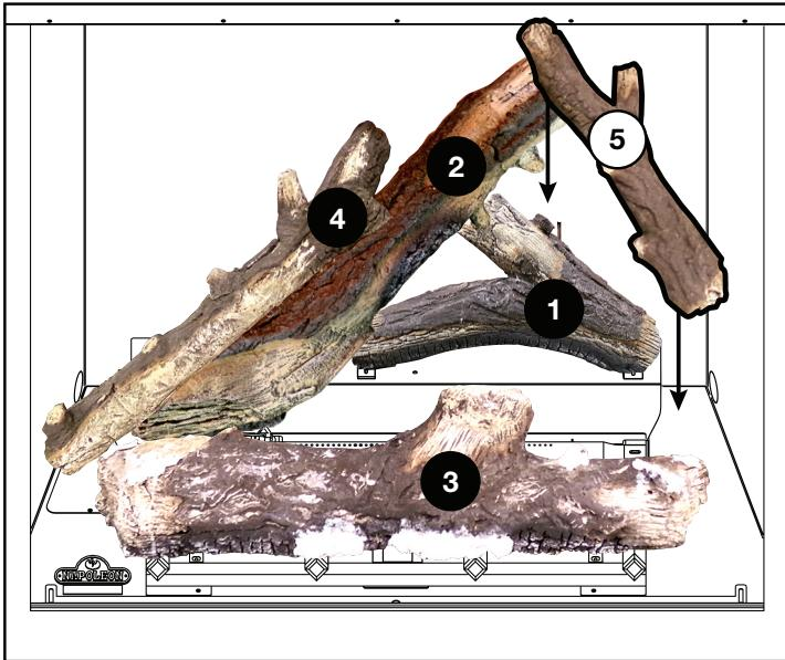
5. Place the locating hole in Log #4 onto the Locating feature on Log #2. Rest the opposite end into the round on the right side of Log #3.
