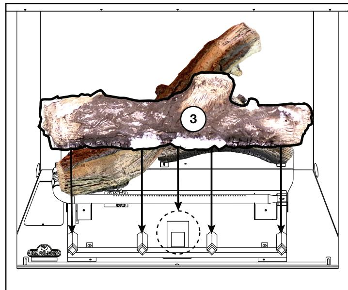
3. Set the round bottom of Log #2 onto the corner of the burner, ensuring the locating knot fits into the hole on the top of Log #1.
