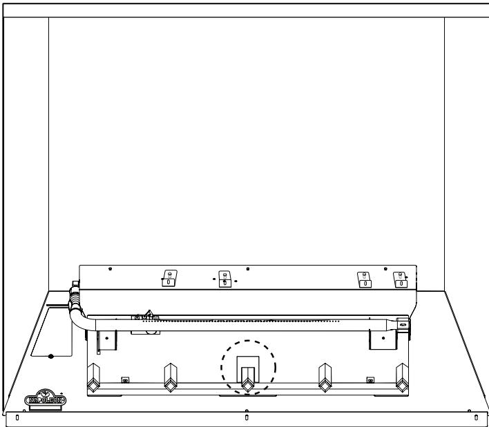
1. Place the Locating Bracket onto the base of the media tray under the middle of the grate. Note: Grate may need loosening.
