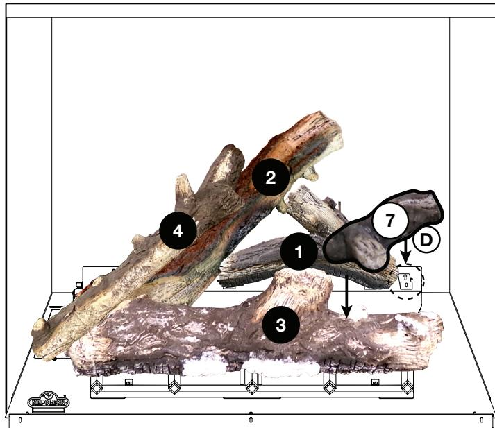
6. Place the locating hole of Log #7 onto locating Stud "D" resting the opposite end onto the locating knot on right side of Log #3.
