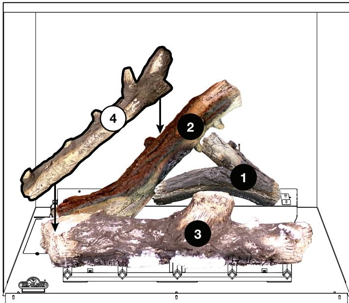
5. Place the locating hole in Log #4 onto the locating feature on Log #2. Resting the opposite end into the round on the right side of Log #3.
