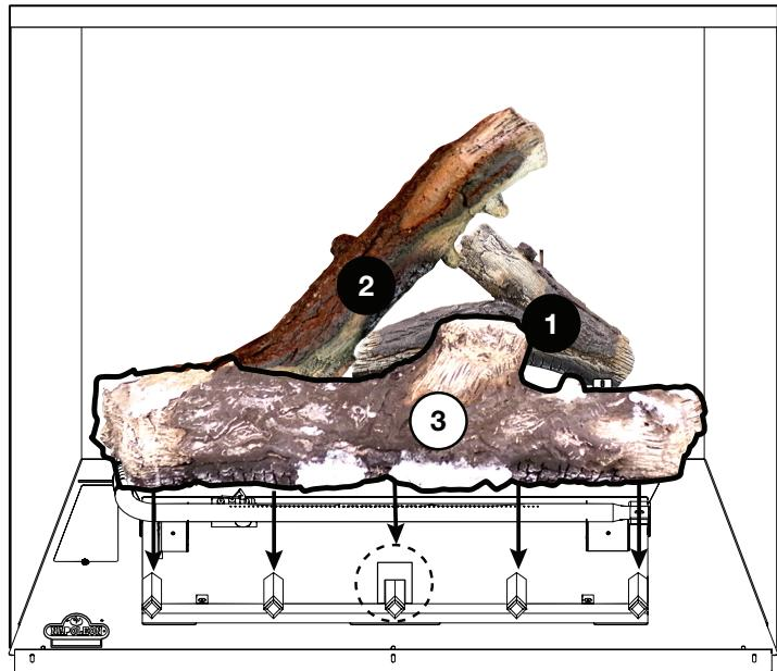
4. Place Log #3 onto the locating bracket installed earlier. Ensure log is sitting on the grate.
