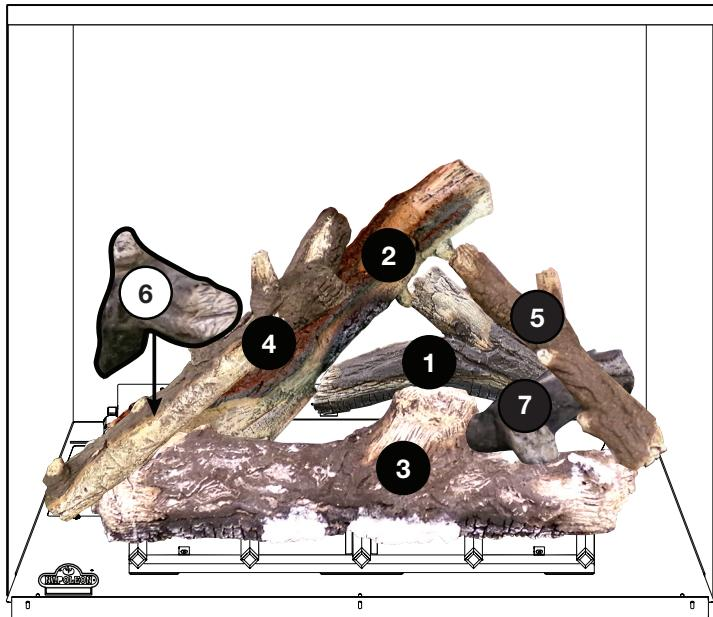
8. Place the locating hole of Log #6 onto the locating knot of Log #4 resting the opposite end onto the media tray.
