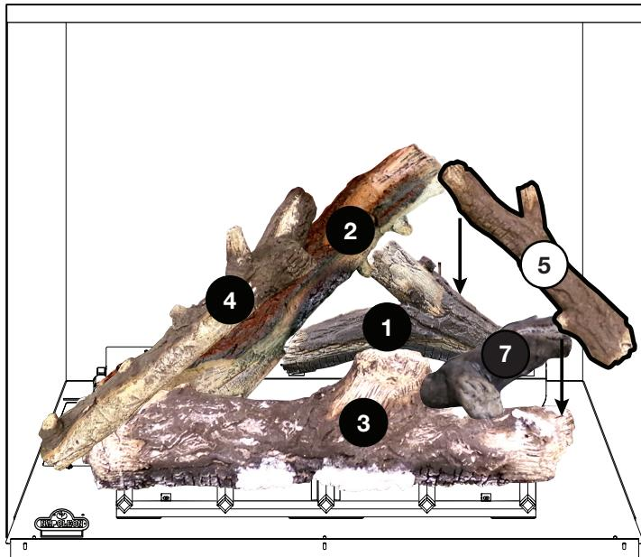
7. Place the locating hole of Log #5 onto locating feature of Log #1 resting the opposite end onto right side of Log #3.
