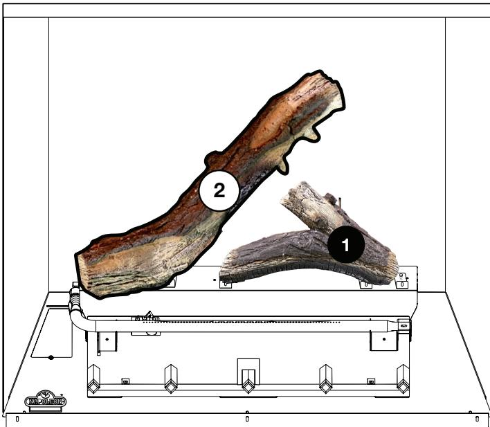
3. Place the round in the bottom of Log# 2 onto the corner of the burner. Resting the locating knot into the locating hole on the top of Log #1.
