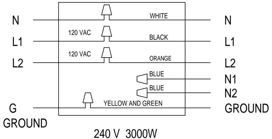
**IF THE APPLIANCE IS TO BE HARD WIRED IN, THE POWER CORD MUST BE REMOVED (SEE INSTRUCTION #1 ON PAGE 20)**
