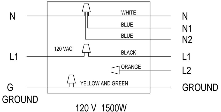
**IF THE APPLIANCE IS TO BE HARD WIRED IN, THE POWER CORD MUST BE REMOVED (SEE INSTRUCTION #1 ON PAGE 20)**
