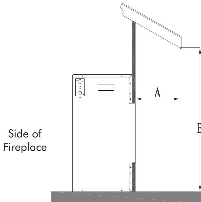
The overhang (A) must extend at least 1/2 the roof-line height (B). Height is measured from the base of the fireplace.
