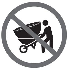
NEVER attempt to move unit in wheelbarrow or other unbalanced equipment that could damage the unit.
