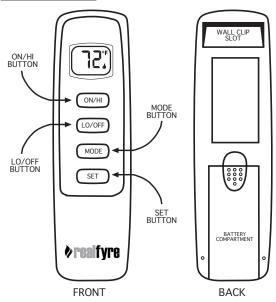
This remote control SYSTEM offers the user a battery-operated remote control to power up to a 6 VDC servo motor or solenoid such as those used with gas valves used in some heater rated gas logs, gas fireplaces and other gas heating appliances.
