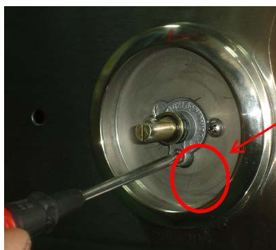
Low flame setting screw (shown for RON series)
