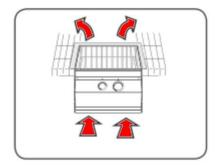
If installed under a patio roof, the cooking grid area should be fully covered by a chimney and exhaust hood. An exhaust fan with a rating of up to 1,000 CFM (472 liters per second) may be necessary to efficiently remove smoke and other Cooking byproducts from the covered area. Installation in fully enclosed patio areas is not recommended.
