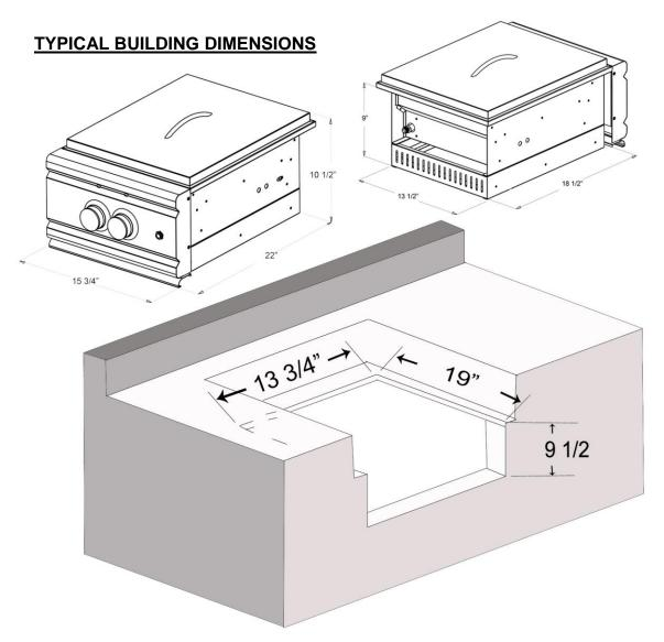
**NOTE:** Its is recommended to build the Pro Burner at least 6"-12" lower than the countertop
