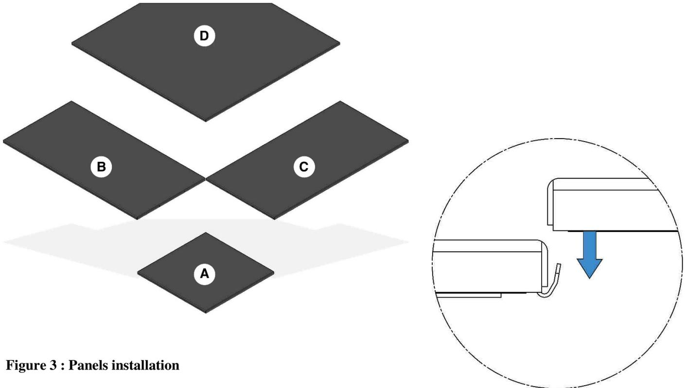
Figure 3 : Panels installation
