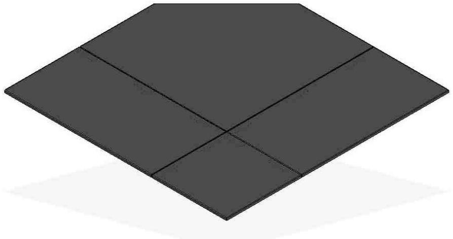
7. Make sure the panels are placed inside one another correctly to protect the floor from hot embers that could fall from the appliance in between two panels that are not well fit together.
